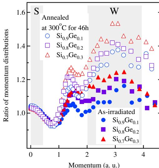
**Figure 4.2.** *Coincidence Doppler broadening results from irradiated  $Si_{1-x}Ge_x$  before and after the annealing treatment.*
