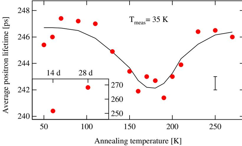
**Figure 5.2.** Average positron lifetime as a function of annealing temperature in Ge after proton irradiation at 35 K. The insert shows the average lifetimes at room temperature after 14 and 28 days. All measurements except the ones in the insert were done at 35 K.
