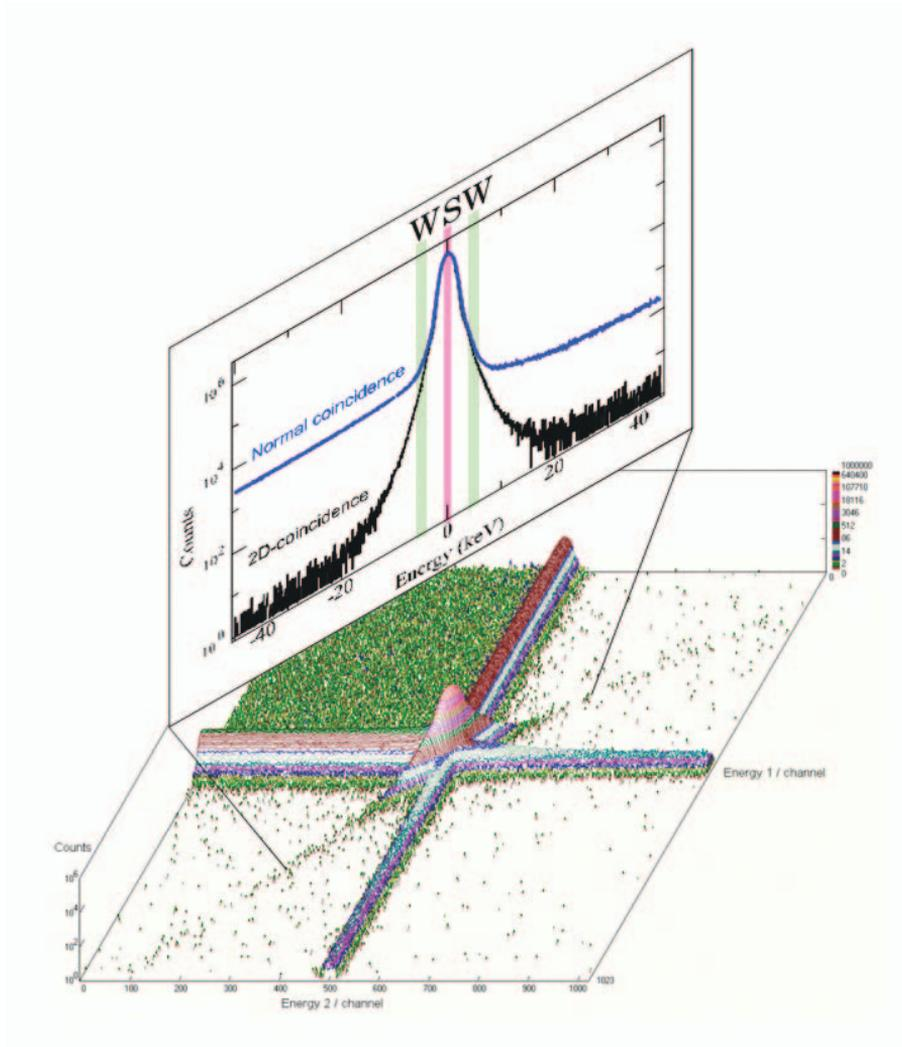
**Figure 3.2.** A two-dimensional Doppler spectrum obtained from a coincidence measurement, and the conventional one-dimensional spectrum obtained from it. Typical  $S$  and  $W$  parameter windows are also presented in the 1-D spectrum.
