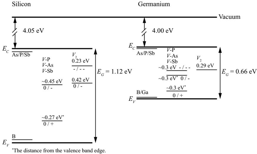
**Figure 2.1.** Ionization level positions of some common defects in the Si and Ge band gaps. The values refer to the distance from the conduction band edge  $E_C$ , except when a value is marked with an asterisk in which case it refers to the distance from the valence band edge  $E_V$ . The exact positions of the vacancy-donor defects depend on the donor atom type. The data is from Refs. [42–45].
