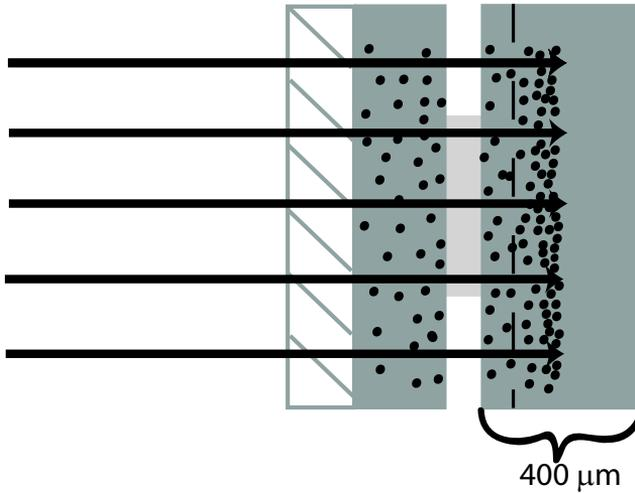
**Figure 5.1.** Schematic of the sample sandwich used in the measurements. The positron source was placed between two sample pieces, one of which was ground to  $\sim 250 \mu\text{m}$ . The grinding was done to avoid positrons from reaching the end-of-range voids in the inner sample piece. The irradiation damage is shown with black dots and the dashed line is drawn to visualize the mean implantation depth of the positrons
