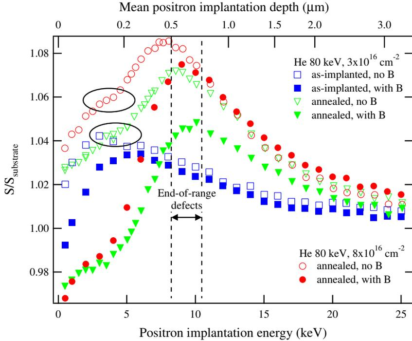
**Figure 5.4.** The  $S$  parameter in the He-implanted samples with implantation fluences of  $3 \times 10^{16} \text{ cm}^{-2}$  and  $8 \times 10^{16} \text{ cm}^{-2}$  (only in annealed samples) as a function of positron implantation energy.
