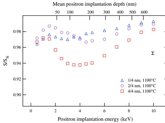
**Figure 6.3.**  $S$  parameters as a function of positron implantation energy for samples with three different Si layer thicknesses annealed in  $N_2$  at  $1100^\circ C$ . The values have been scaled to that of defect-free bulk Si.
