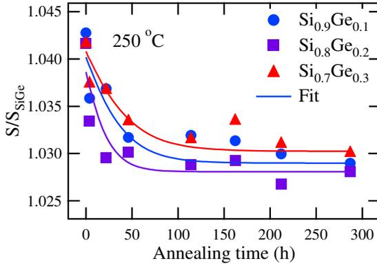
**Figure 4.1.** Measured (markers) and fitted (lines)  $S$  parameters from  $Si_{1-x}Ge_x$  annealed at  $250^\circ C$ . The starting points at 0 hours correspond to "as-irradiated" values associated with  $E$  centers.
