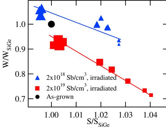
**Figure 4.6.**  $S, W$  parameters measured in  $\text{Si}_{0.8}\text{Ge}_{0.2}$  samples isochronally annealed at 30 minute steps. Increasing symbol size emphasizes increasing annealing temperature. The values have been scaled to those of as-grown  $\text{Si}_{0.8}\text{Ge}_{0.2}$ .
