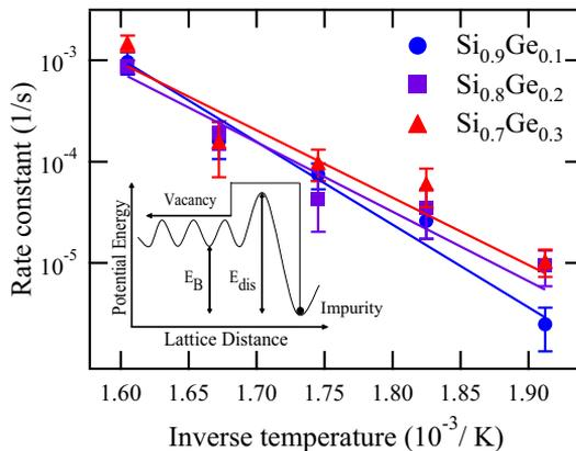
**Figure 4.4.** Arrhenius plot for the annealing rate constant. The slope of the lines fitted to the experimental data points is interpreted as the dissociation energy for the diffusion of the  $E$  center in  $\text{Si}_{1-x}\text{Ge}_x$ . The insert shows a schematic representation of the dissociation ( $E_{dis}$ ) and binding ( $E_B$ ) energies of the vacancy-impurity pair.
