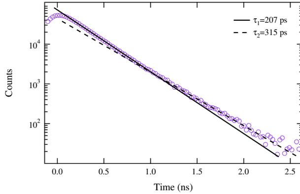
**Figure 3.1.** *Positron lifetime spectrum of proton irradiated Ge measured at RT. The lines are fits of the two positron lifetime components found in the experimental data.*
