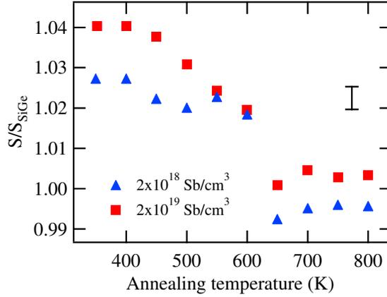
**Figure 4.5.**  $S$  parameter as a function of annealing temperature in samples isochronally annealed at 30 minute steps. The values are scaled to those of as-grown  $Si_{0.8}Ge_{0.2}$ . The typical error margin of the parameters is also included.
