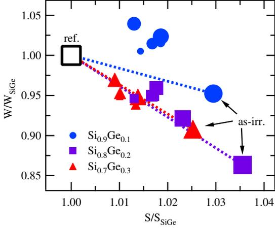
**Figure 4.3.**  $(S,W)$  parameters of irradiated and annealed  $Si_{1-x}Ge_x$  layers with varying Ge contents. The data shown are the final points of each annealing series. Decreasing symbol size visualizes an increase in annealing temperature. Values from each sample are scaled to the respective bulk
