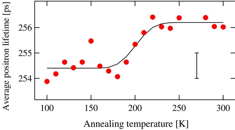
**Figure 5.3.** Average positron lifetime as a function of annealing temperature in Ge after proton irradiation at 100 K. All measurements were performed at 35 K.
