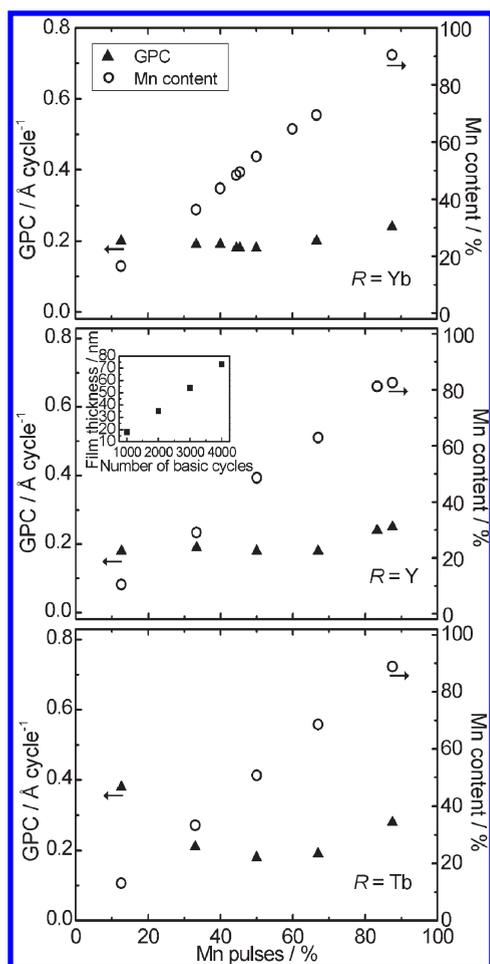
**Figure 1.** Effect of the precursor pulsing ratio on the actual Mn content (○) and the growth-per-cycle (GPC) value (▲) of  $R_xMn_yO_3$  ( $R = Yb, Y, Tb$ ) films at deposition temperature of 275 °C. The inset shows the dependence of the  $Y_xMn_yO_3$  (with a Y/Mn pulsing ratio of 1:1) film thickness on the number of basic ALD cycles.
