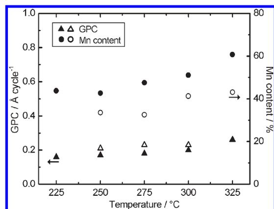
**Figure 2.** Temperature dependencies of the growth-per-cycle (GPC) value (triangles) and the Mn content (circles) for  $R_xMn_yO_3$  ( $R = Y, Tb$ ) deposited with a R/Mn pulsing ratio of 1:1 (the number of basic ALD cycles was 2000). Filled symbols refer to  $Y_xMn_yO_3$  and open symbols to  $Tb_xMn_yO_3$ .
