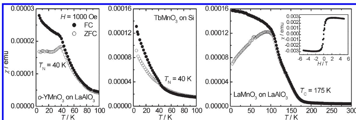
**Figure 6.** Temperature dependence of magnetic susceptibility ( $\chi$ ) in ZFC and FC modes under an external field of 1000 Oe for  $o$ -YMnO<sub>3</sub> on LaAlO<sub>3</sub>, TbMnO<sub>3</sub> on silicon, and La<sub>1-x</sub>Mn<sub>1-x</sub>O<sub>3</sub> on LaAlO<sub>3</sub>. Inset: field dependence of magnetic susceptibility (measured at 5 K) of a La<sub>1-x</sub>Mn<sub>1-x</sub>O<sub>3</sub> film deposited on LaAlO<sub>3</sub>.
