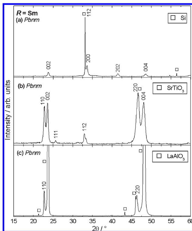
**Figure 4.** XRD patterns for annealed  $\text{SmMnO}_3$  films deposited on (a)  $\text{Si}(100)$ , (b)  $\text{SrTiO}_3(100)$ , and (c)  $\text{LaAlO}_3(100)$  substrates. The indices are for the orthorhombic space group  $Pbnm$ . The film thickness was 200 nm.
