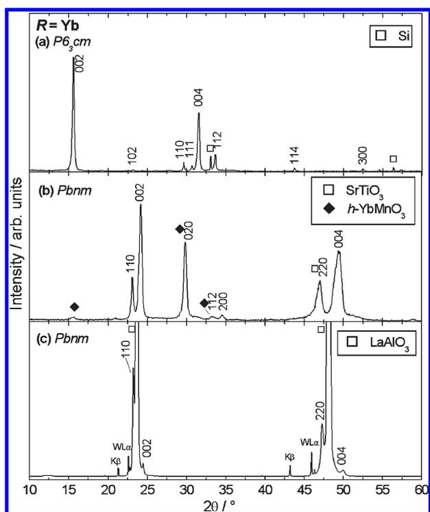
**Figure 3.** XRD patterns for annealed  $\text{YbMnO}_3$  films deposited on (a)  $\text{Si}(100)$ , (b)  $\text{SrTiO}_3(100)$ , and (c)  $\text{LaAlO}_3(100)$  substrates. The indices are for the hexagonal space group  $P6_3cm$  in (a) and for the orthorhombic space group  $Pbnm$  in (b) and (c). The film thickness was 200 nm.
