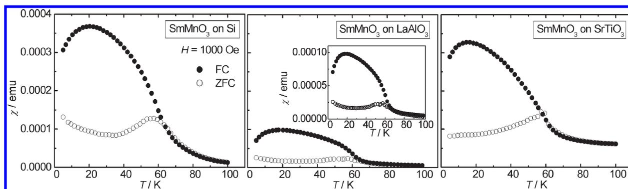
**Figure 5.** Temperature dependence of magnetic susceptibility ( $\chi$ ) in ZFC and FC modes under an external field of 1000 Oe for  $\text{SmMnO}_3$  thin-film samples deposited on silicon,  $\text{LaAlO}_3$ , and  $\text{SrTiO}_3$ .
