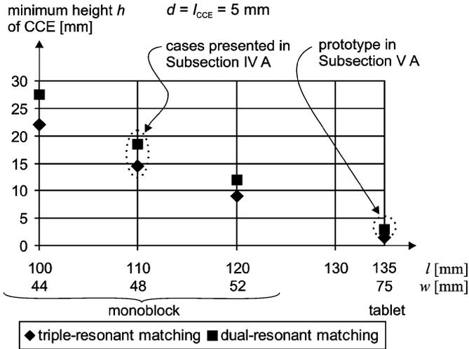
Fig. 11. Effect of different terminal sizes on the minimum height of the coupling element in dual-resonant and triple-resonant matching cases.  $d = l_{CCE} = 5 Pmm$ .
