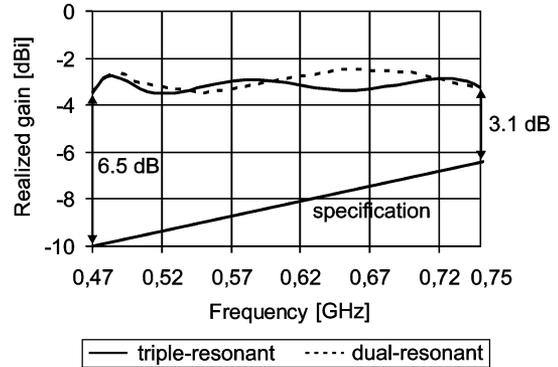
Fig. 8. Simulated realized gains of the example design.
