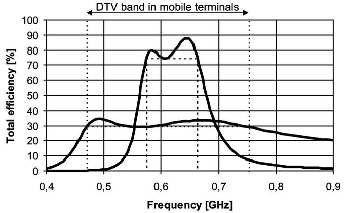
Fig. 2. Conceptual graph on how a narrow-band antenna can be matched so that a larger bandwidth is covered at the expense of the total efficiency.
