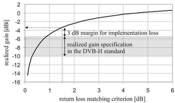
Fig. 3. Realized gain estimation of a DTV antenna as a function of the return loss matching criterion.
