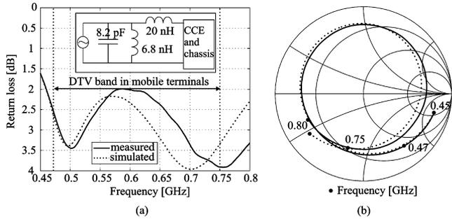
Fig. 15. Simulated and measured return loss of the tablet-size prototype (a) in the Cartesian coordinate system and (b) on the Smith chart.
