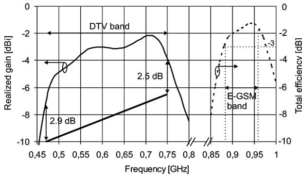
Fig. 20. Simulated realized gain of the DVB-H antenna and the simulated total efficiency of the E-GSM antenna of the typical-size terminal design.
