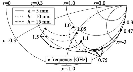
Fig. 4. Impedance curves at 0.3–1.5 GHz when  $h$  is 5, 10, and 15 mm.
