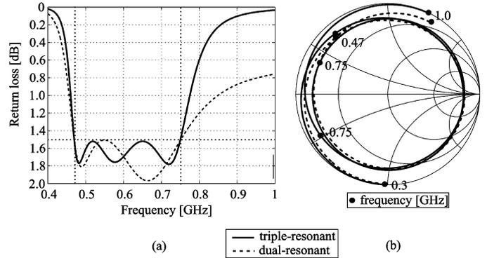
Fig. 7. Simulated (a) return loss in the Cartesian coordinate system and (b) the complex impedance on the Smith chart for the example design.
