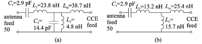
Fig. 6. (a) Triple-resonant and (b) dual-resonant matching circuits and their component values for the example design.
