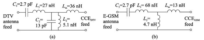
Fig. 18. Matching circuits for simulated (a) DTV and (b) E-GSM antennas.
