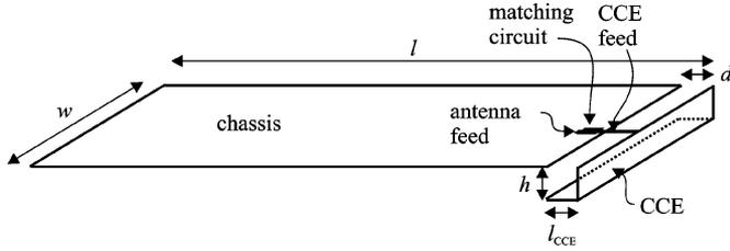
Fig. 1. Capacitive coupling element (CCE) structure.
