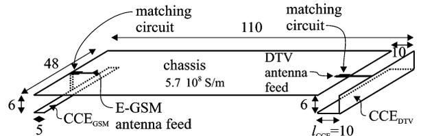
Fig. 17. Structure of the simulated design for typical-size terminal. Dimensions are in mm.
