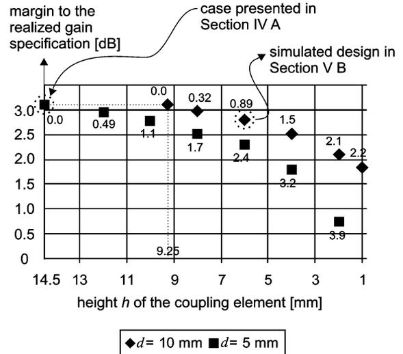
Fig. 13. Minimum margin to the realized gain specification versus the height of the element (triple-resonant matching) for typical-size monoblock.  $x \cdot x \Omega$  is the resistance of the resistor added between the antenna element and the matching circuit.
