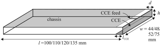
Fig. 10. Minimum outer dimensions of the different-size terminals. Gray color illustrates the capacitive coupling element and the chassis. The sketch is not in the real scale.
