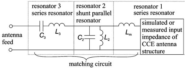
Fig. 5. General triple-resonant matching circuit with series and parallel resonators in turn.
