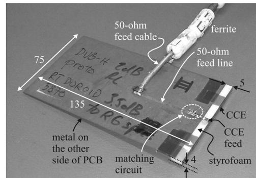
Fig. 14. Photograph of the tablet-size DTV prototype. The shape and dimensions (in mm) of the antenna are similar to shown in Fig. 10.
