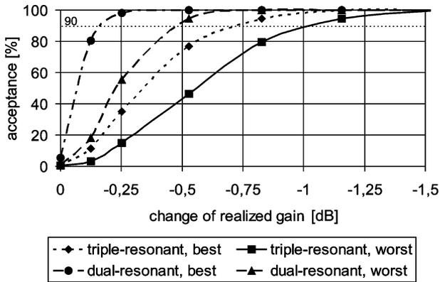
Fig. 9. Effect of the variation of the matching circuit component values on the realized gain.
