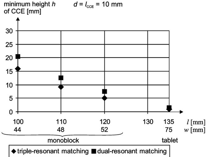
Fig. 12. Effect of different terminal sizes on the minimum height of the coupling element in dual-resonant and triple-resonant matching cases.  $d = l_{CCE} = 10$  mm.
