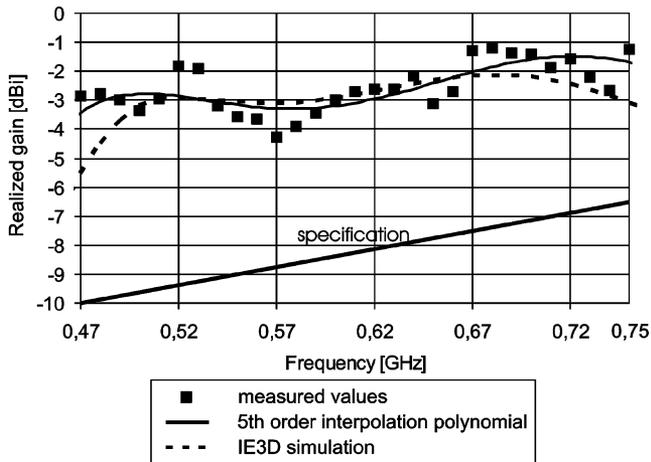
Fig. 16. Simulated and measured realized gain of the tablet-size DTV prototype.
