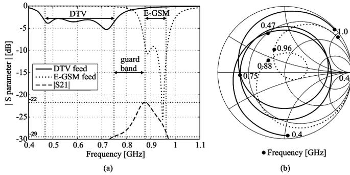
Fig. 19. Simulated  $S$  parameters of the typical-size terminal design (a) in the Cartesian coordinate system and (b) on the Smith chart.
