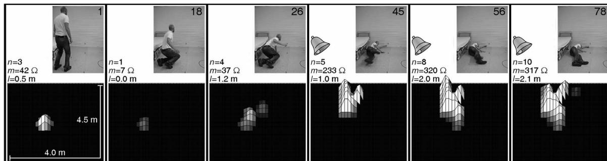
Fig. 2. Example of fall detection with the NFI floor sensor. Video (30 fps) and NFI data were recorded simultaneously. The bell indicates the fall-alarm state.
