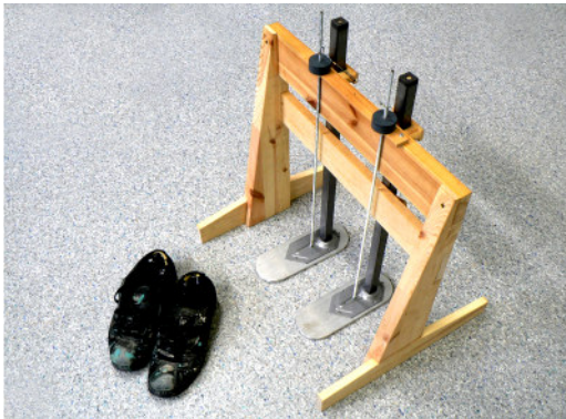
Figure 2 The Human body phantom with adjustable legs. European foot size is 41. Leg to leg Impedance is 500 \Omega . Test shoes used in the tests had 15 mm thick synthetic rubber soles. Sensor array is under a plastic floor covering.
