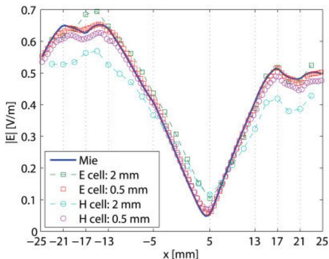
**Figure 6** Electric field amplitude along the diagonal of the 5-layer sphere at 1 GHz. [Color figure can be viewed in the online issue, which is available at [www.interscience.wiley.com](http://www.interscience.wiley.com)]
