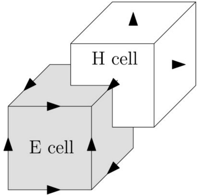
**Figure 1** Positioning of the electric field components in the E-cell and H-cell grids
