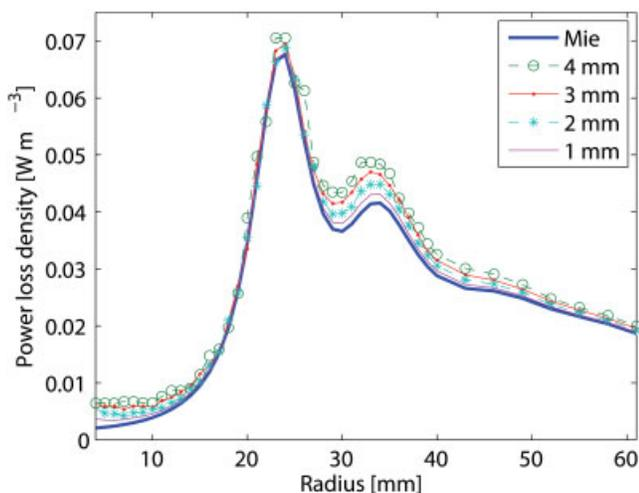
**Figure 4** Average power loss density as a function of sphere radius at various resolutions when the materials are positioned in E cells. [Color figure can be viewed in the online issue, which is available at [www.interscience.wiley.com](http://www.interscience.wiley.com)]
