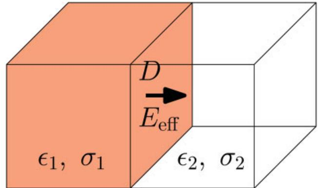
**Figure 3** Position of the electric field component on the interface of two H cells. [Color figure can be viewed in the online issue, which is available at [www.interscience.wiley.com](http://www.interscience.wiley.com)]
