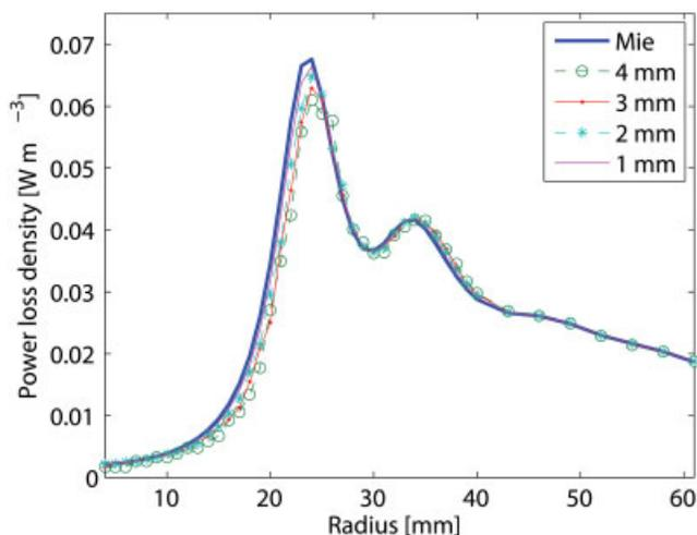
**Figure 5** Average power loss density as a function of sphere radius when the materials are positioned in H cells. [Color figure can be viewed in the online issue, which is available at [www.interscience.wiley.com](http://www.interscience.wiley.com)]
