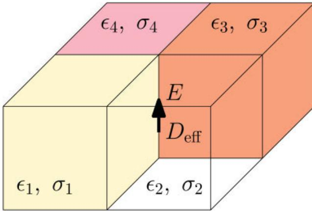
**Figure 2** Electric field component in the intersection of four E cells. [Color figure can be viewed in the online issue, which is available at [www.interscience.wiley.com](http://www.interscience.wiley.com)]
