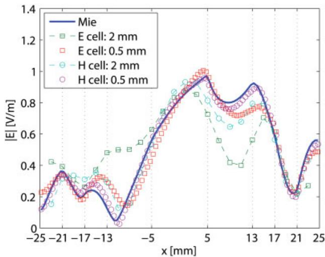
**Figure 7** Electric field amplitude along the diagonal of the 5-layer sphere at 2.5 GHz. [Color figure can be viewed in the online issue, which is available at [www.interscience.wiley.com](http://www.interscience.wiley.com)]
