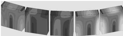
Fig. 7. The eddy current loss density in (the halves of) 30 mm long magnets with sinusoidal input of 3 kHz (tenth harmonic of the converter input frequency).
