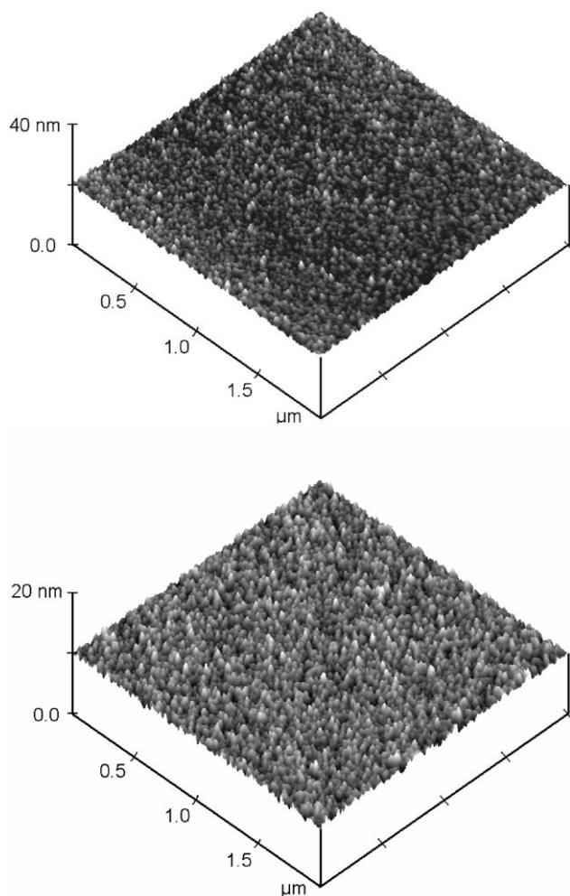
**Fig. 5** Representative AFM images of  $\text{Er}_x\text{Ga}_{2-x}\text{O}_3$  thin films deposited by ALD using  $\text{Er}(\text{C}_5\text{H}_4\text{Me})_3$ ,  $\text{Ga}_2(\text{NMe}_2)_6$ , and water with an erbium : gallium pulse ratio of 1 : 1 (top; film thickness = 57 nm) and  $\text{Er}(\text{thd})_3$ ,  $\text{Ga}(\text{acac})_3$ , and ozone with an erbium : gallium pulse ratio of 11 : 5 (bottom; film thickness = 46 nm). The measured rms values were 0.6 nm and 0.4 nm, respectively.
