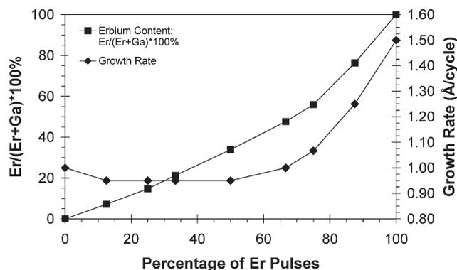
**Fig. 2** Film composition and growth rate plotted as a function of the precursor pulse ratio (expressed as the percentage of the total number of metal precursor pulses that were erbium precursor pulses) for the  $\text{Er}(\text{C}_5\text{H}_4\text{Me})_3$ ,  $\text{Ga}_2(\text{NMe}_2)_6$ , and water process.
