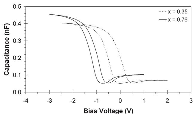
**Fig. 7** Capacitance–voltage curves of  $\text{Al}/\text{Er}_x\text{Ga}_{2-x}\text{O}_3/\text{SiO}_2/\text{p-Si}(100)$  capacitor structures with an  $\text{Er}_x\text{Ga}_{2-x}\text{O}_3$  film grown at  $250^\circ\text{C}$  from  $\text{Er}(\text{C}_5\text{H}_4\text{Me})_3$ ,  $\text{Ga}_2(\text{NMe}_2)_6$ , and water. For  $x = 0.35$  and 0.76, the film thicknesses were 41.4 and 42.6 nm, respectively.
