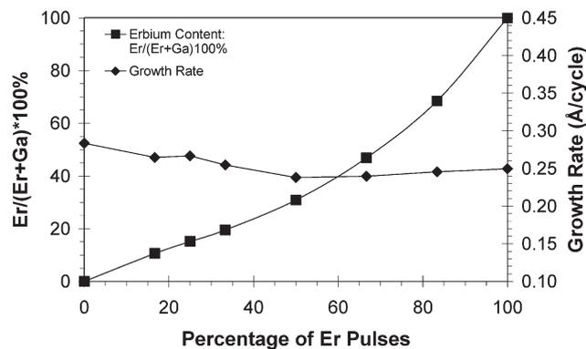
**Fig. 1** Film composition (as determined by XRF) and growth rate plotted as a function of the precursor pulse ratio (expressed as the percentage of the total number of metal precursor pulses that were erbium precursor pulses) for the  $\text{Er}(\text{thd})_3$ ,  $\text{Ga}(\text{acac})_3$ , and ozone process.
