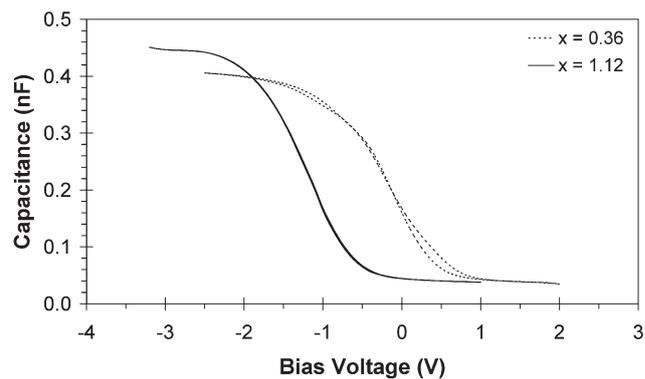
**Fig. 6** Capacitance–voltage curves of  $\text{Al}/\text{Er}_x\text{Ga}_{2-x}\text{O}_3/\text{SiO}_2/\text{p-Si}(100)$  capacitor structures with an  $\text{Er}_x\text{Ga}_{2-x}\text{O}_3$  film grown at  $350^\circ\text{C}$  from  $\text{Er}(\text{thd})_3$ ,  $\text{Ga}(\text{acac})_3$ , and ozone. For  $x = 0.36$  and 1.12, the film thicknesses were 48.6 and 45.6 nm, respectively.
