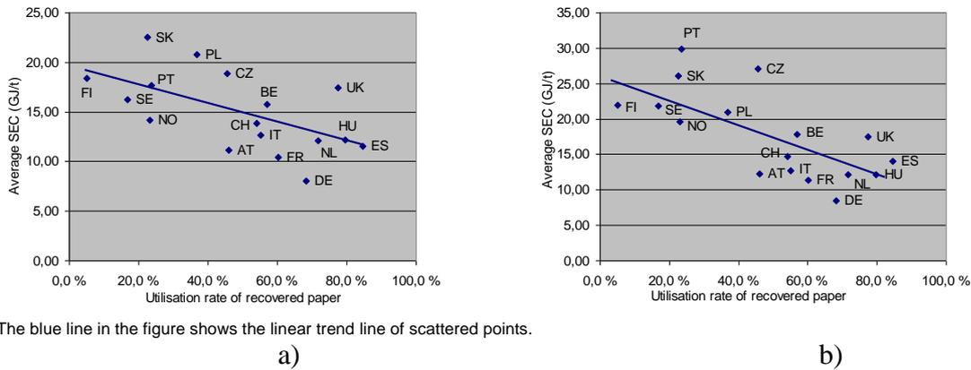
**Figure 7.** The influence of the utilisation rate of recovered paper on the average SEC a) the SEC calculated for paper and market pulp production [23, 24] b) the SEC calculated for paper production [23, 25].
