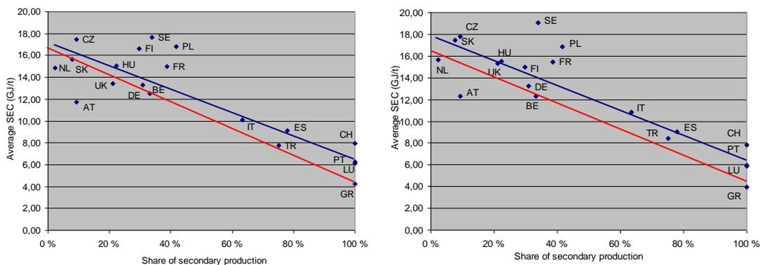
The upper blue line in the figures shows the linear trend line of scattered points and the lower red line the theoretical curve between the world best practice final energy intensity values of primary production and secondary production (for continuous casting and hot rolling of bars).
