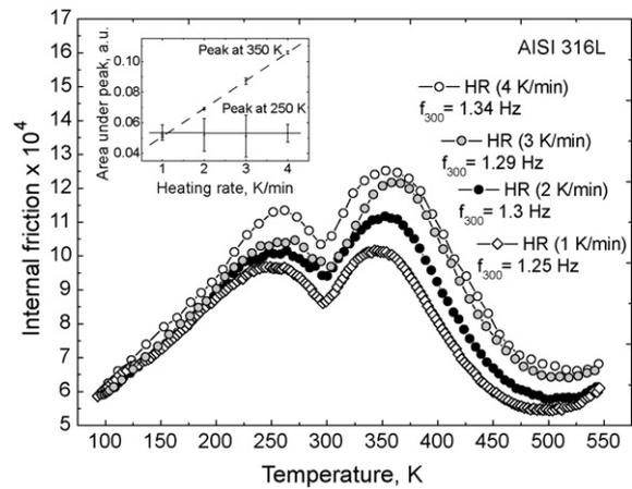
**Fig. 3.** Temperature dependence of internal friction of AISI 316L steel at different heating rates. The inset shows the dependence of the area under fitted peaks on heating rate for the low- (dashed line) and the high-temperature peak (solid line).
