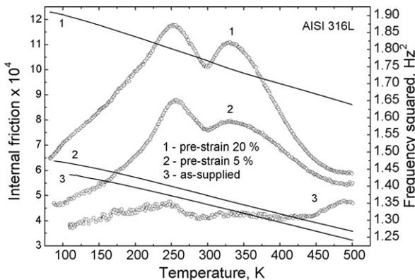
**Fig. 2.** Change of the peaks in AISI 316L austenitic stainless steel plastically pre-strained in tension at room temperature and at a strain rate of  $10^{-3} \text{ s}^{-1}$ .
