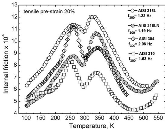
**Fig. 1.** Temperature dependence of internal friction for different grades of austenitic stainless steels after prior plastic deformation in tension to 20% strain at room temperature and at a strain rate of  $10^{-3} \text{ s}^{-1}$ .
