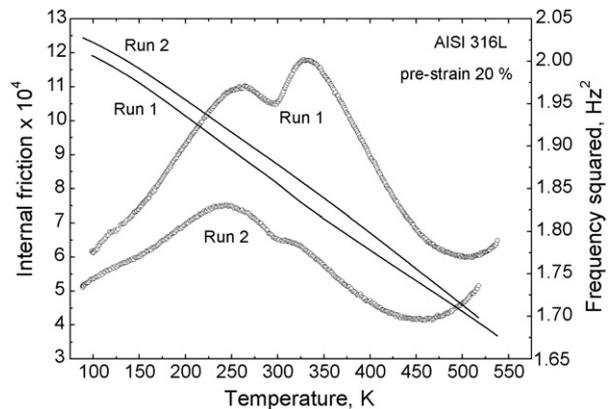
**Fig. 4.** Temperature dependence of internal friction and squared natural frequency for AISI 316L austenitic stainless steel after tensile pre-strain of 20% at room temperature and at a strain rate of  $10^{-3} \text{ s}^{-1}$ . Comparison between data of the first and second measurement runs.
