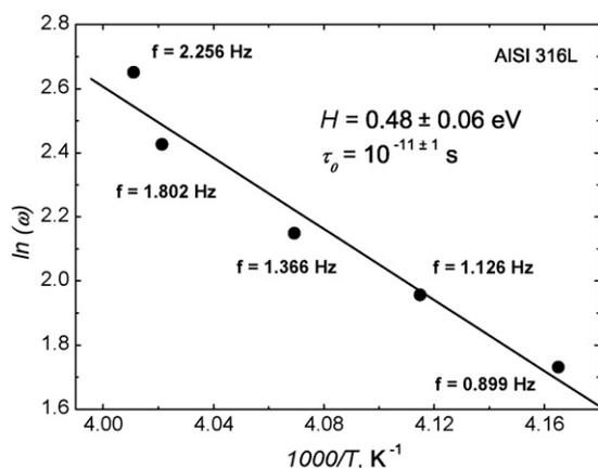
Fig. 5. Arrhenius plot for the low-temperature peak P1, obtained after removal of transitional high-temperature peak P2 by annealing at 550 K for 100 min.
