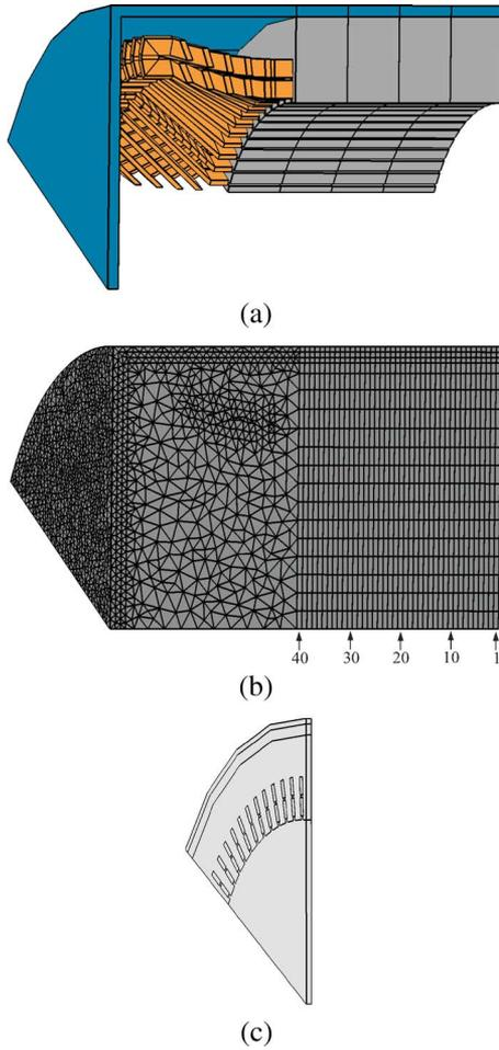
Fig. 1. The 3-D model of the simulated machine: (a) the geometric model (without the air region); (b) the finite element mesh of the model with the indexes of the slices; and (c) one of the slices of the model for the calculation.
