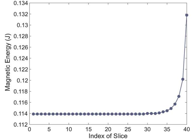
Fig. 3. Arithmetic mean value of the magnetic energy in each slice of the model at the rated frequency.
