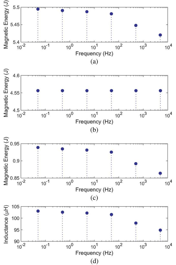
Fig. 5. Analysis of the stator end-winding leakage inductance under different excitation frequencies, 0.05 Hz, 0.5 Hz, 5 Hz, 50 Hz, 500 Hz, and 5000 Hz: (a)  $\overline{W}_{m,tot}$ ; (b)  $\overline{W}_{m,act}^{src}$ ; (c)  $\overline{W}_{m,end}^{src}$ ; and (d)  $L_{\sigma,end}^{str}$ .
