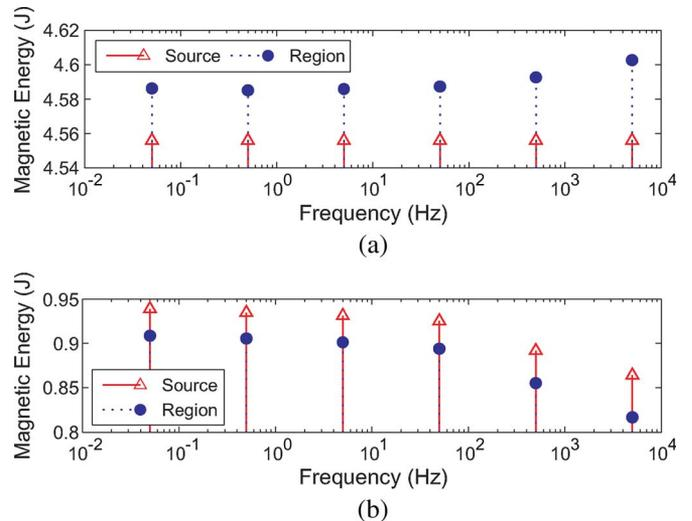
Fig. 6. The comparison of different components of the magnetic energy under different excitation frequencies, 0.05 Hz, 0.5 Hz, 5 Hz, 50 Hz, 500 Hz, and 5000 Hz: (a)  $\overline{W}_{m,act}^{src}$  and  $\overline{W}_{m,act}^{reg}$  and (b)  $\overline{W}_{m,end}^{src}$  and  $\overline{W}_{m,end}^{reg}$ .
