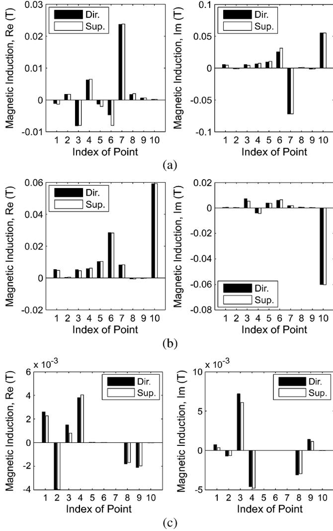
Fig. 2. Real and imaginary parts of the magnetic induction at 10 spatial points by the direct solution and by the superposition method: (a)  $x$ -component; (b)  $y$ -component; and (c)  $z$ -component.
