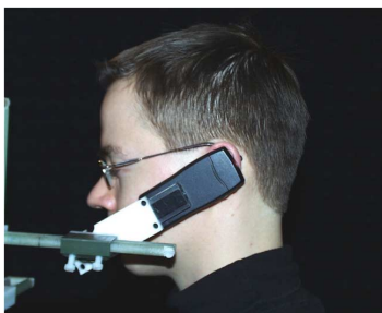
Fig. 2. One of the test persons in set-up c) during the first measurement campaign. In this setup, the test person did not hold the DUT with the hand, but the DUT was next to the head using a plastic fixture.
