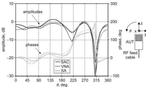
**Fig. 2** Comparison of amplitude and phase pattern of  $\theta$  component of radiated far field in  $y$ - $z$  plane obtained by SA, VNA, SAC measurements
