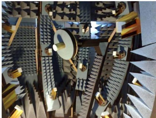
Fig. 4. Measurement of the TZF. The TZF probe is measured in different orientations in the test zone.
