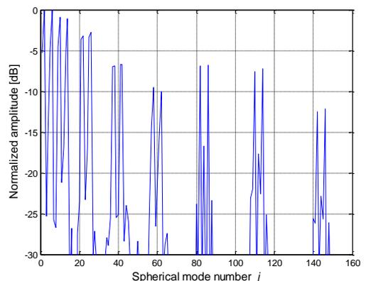
Fig. 2. The spherical mode spectrum of the TZF probe at 1.6 GHz.
