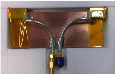
Fig. 3. The diversity antenna prototype (AUT1 & AUT2).
