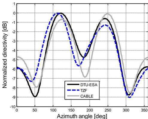
Fig. 5. A representative pattern cut for AUT1, showing the DTU-ESA reference measurement and the TKK measurement with TZF and cable calibration.
