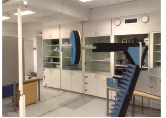
Fig. 2. Test zone field measurement with a calibration antenna.
