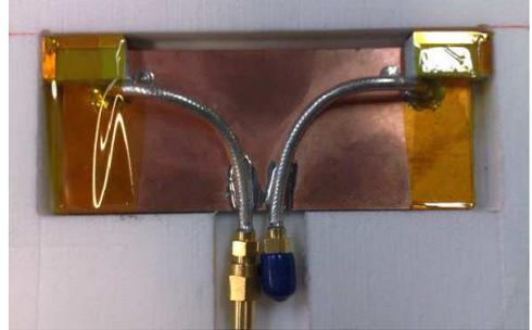
Fig. 7. Diversity antenna structure as AUT.
