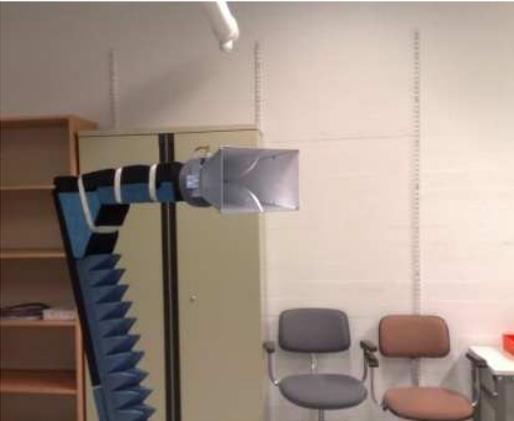
Fig. 4. Measurement of AUT1 in a laboratory room with no RF-absorber coating on the walls.
