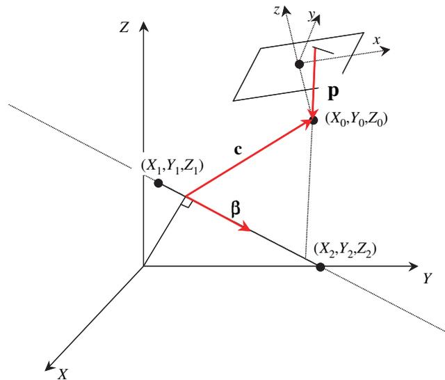
FIG. 3. Coplanarity model used in line photogrammetry.
