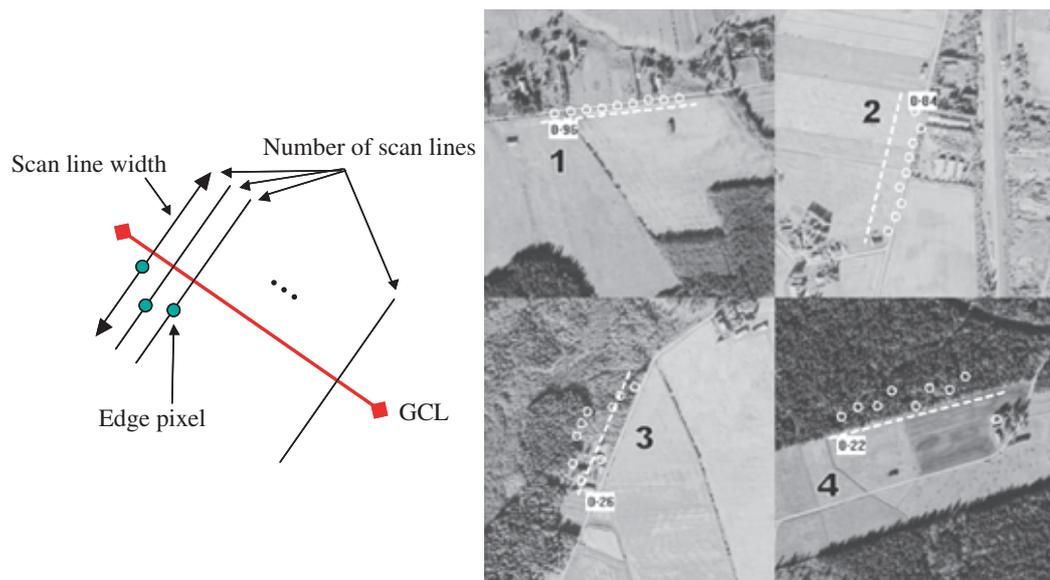
FIG. 2. Idea of local line scanning and four example cases.
