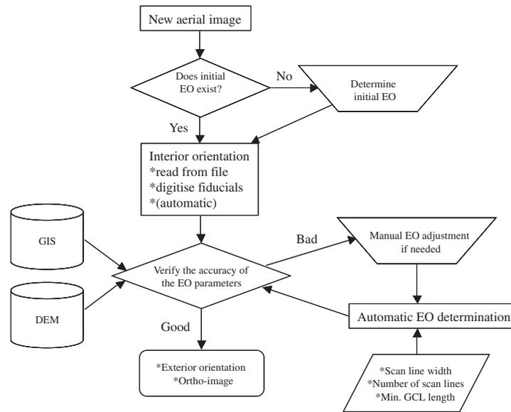
FIG. 1. Flow chart of EO procedure.
