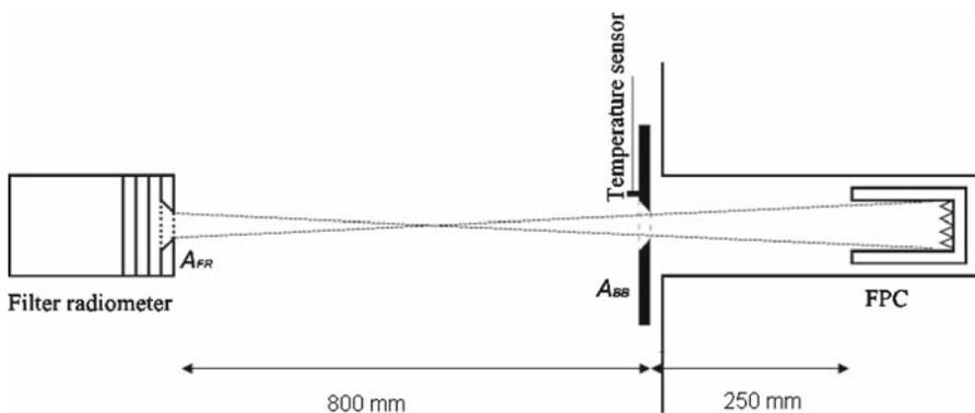
**Fig. 1** Setup used for fixed-point cell (FPC) and variable-temperature blackbody (VTBB) measurements.  $A_{\text{FR}}$  is the filter radiometer aperture area, and  $A_{\text{BB}}$  is the defining area for the blackbody
