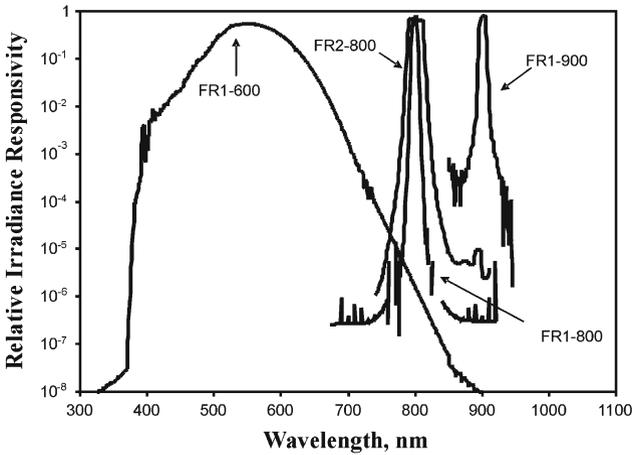
**Fig. 2** Spectral responsivities of the filter radiometers
