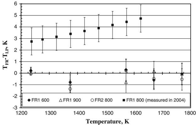
**Fig. 4** Differences of the variable-temperature blackbody temperatures measured with a filter radiometer and the pyrometer in 2004 and in 2006. For the 2006 measurements, filled diamonds, open triangles, and open circles correspond to FR1-600, FR1-900, and FR2-800 data, respectively. Standard uncertainties ( $k = 1$ ) associated with the comparison of the filter radiometer and pyrometer are indicated
