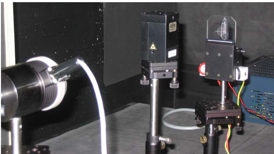
Figure 7. Alignment of the filter radiometer and an FEL lamp. Devices from left to right: Filter radiometer, alignment laser, lamp with an alignment target and power supply.
