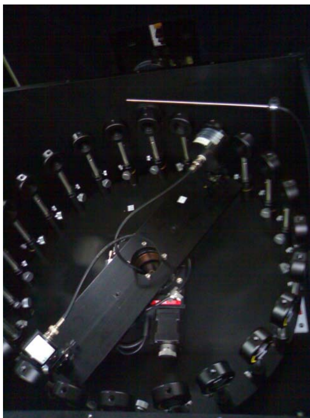
Figure 9. The MWFR facility of NMC. The Si and InGaAs detectors are placed on the central rotary stage. The 24 filters are placed on the outermost rotary stage.
