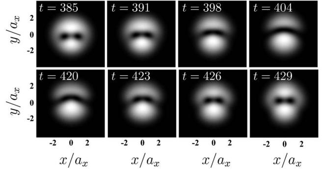
FIG. 4. Collapse and revival of the slightly perturbed stationary vortex dipole state for  $\tilde{g}=60$  and  $\lambda=1$ . It should be noted that apart from oscillations of the vortex locations, the vortex dipole state remains essentially intact for a long time before it starts to decay. The vortices have opposite topological charges after the revival of the dipole state.
