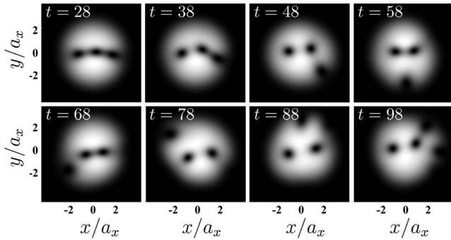
FIG. 5. Temporal evolution of the perturbed stationary vortex triple state for  $\tilde{g}=160$  and  $\lambda=1$ . The vortex triple starts to decay almost immediately to the vortex dipole state due to the strong dynamical instability.
