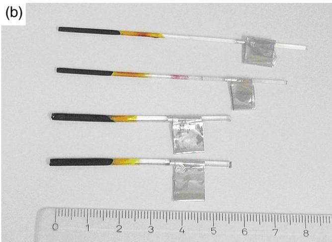
Fig. 2. (a) Schematic drawing of the PV fiber. (b) Photograph of the PV fibers (without the CE contacts) of different diameters.
