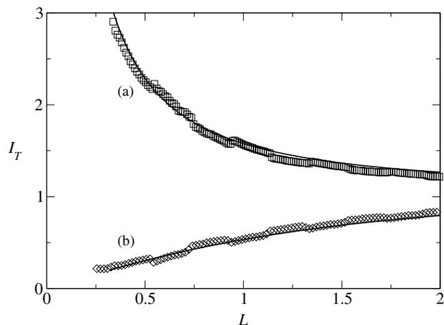
Fig. 4. Feedback approach curves for (a) 0.5 mM  $\text{Ru}(\text{bipy})_3^{2+}$  at an nSi/dsDNA surface and (b) 1 mM  $\text{Co}(\text{bipy})_3^{3+}$  at a pSi/dsDNA surface. The electrolyte was 20 mM Tris buffer at pH 7.5 and the tip radius was 5  $\mu\text{m}$ . The tip potential was (a) 1.15 V vs. SCE and (b) 0.05 V vs. SCE. The solid lines are the curves for diffusion controlled positive feedback (metallic behaviour) and pure negative feedback (insulator behaviour).
