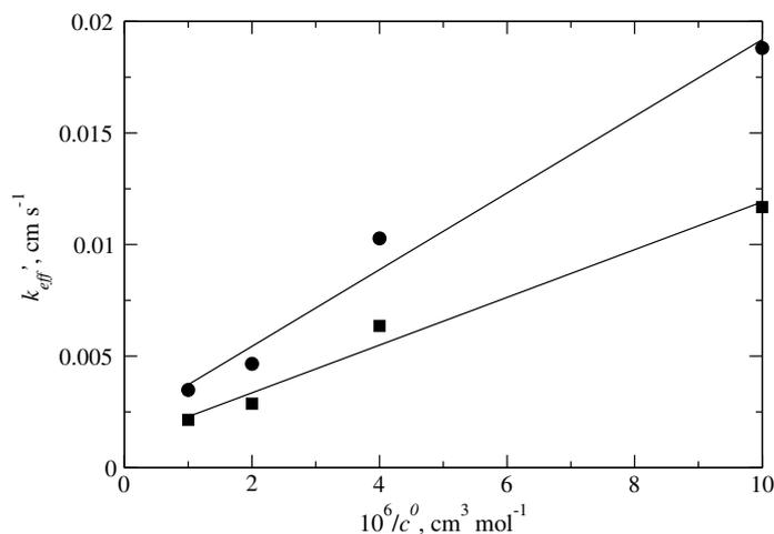
Fig. 8. Plot of  $k_{\text{eff}}$  vs.  $1/c^0$  according to Eq. (9) for  $\text{Ru}(\text{NH}_3)_6^{3+}$  at pSi/dsDNA surfaces as a function of bulk solution concentration. The electrolyte was 20 mM Tris buffer at pH 7.5 and the tip radius was 5  $\mu\text{m}$ . Since  $k_{\text{eff}}$  depends on the distance, two representative values were chosen, i.e.,  $d = 0.5a$  (circles) and  $d = 1.0a$  (squares). The lines are least-squares fits as guides to the eye.
