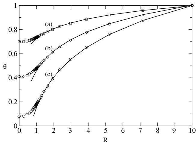
Fig. 12. Typical plots of normalised surface coverage ( $\theta = \Gamma/\Gamma^*$ ) versus radial distance in units of tip radius ( $R$ ) from the finite difference simulation. The solid lines show the behaviour used in the analytical approximation, Eq. (13). (a)  $\zeta=6.4$ , (b)  $\zeta=2.0$  and (c)  $\zeta=0.21$ .
