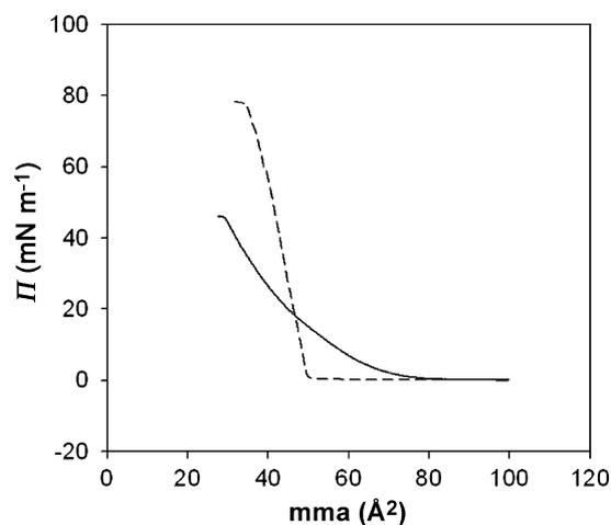
**Fig. 3** – Isotherms measured at the air/water interface for a DPPC lipid monolayer with 10% DPPS (solid line) and a DSPC lipid monolayer (dashed line).
