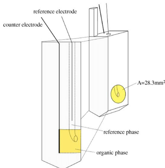
**Fig. 1 – A schematic illustration of the electrochemical cell used in this study.**
