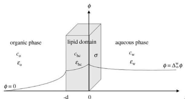
**Fig. 2 – Boundary conditions for the potential distribution.**  $c_o$ ,  $c_w$  and  $c_{hc}$  refer to concentrations in the organic phase, aqueous phase and lipid domain, respectively and  $\epsilon_o$ ,  $\epsilon_w$ ,  $\epsilon_{hc}$  refer to permittivity of these domains.  $\sigma$  represents the surface charge of the monolayer.
