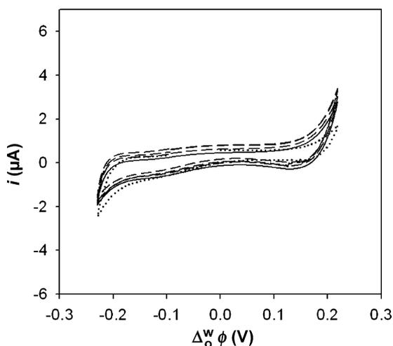
**Fig. 4** – CVs obtained at the lipid modified NPOE–water interface in the presence of supporting electrolytes (dotted line), ODN2 naked (solid line) and ODN2 complexed with different ratios of surfactant (dashed lines).
