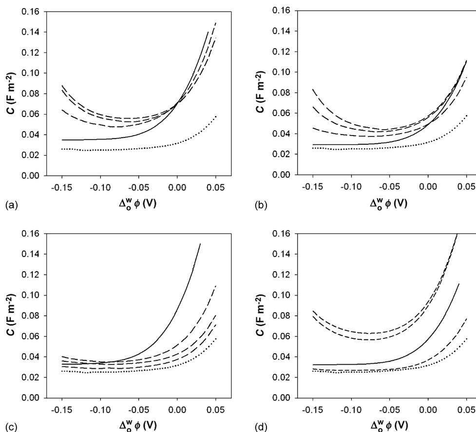
**Fig. 7 – Theoretical capacitance curves: (A) ODN1.** The solid line shows the predicted response for the case of the naked oligonucleotide and the dashed lines show the responses for the complexed oligonucleotides with the CP/oligonucleotide ratios of 0.24, 0.71 and 0.96 from bottom to top. The dotted line shows the response predicted for the compressed lipid monolayer with only base electrolytes in aqueous compartment, (B) ODN2, (C) MOD1 and (D) MOD2. The lines are assigned as in (A).
