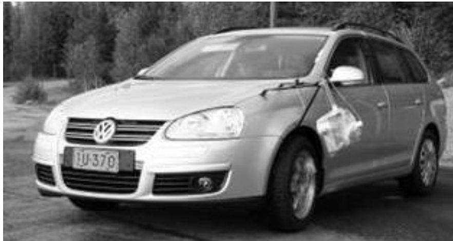
Figure 4 Measurement vehicle and tyre sensor (front left) with the radio receiver
