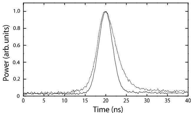
Fig. 4. Oscilloscope traces of pulses at 561 nm (solid) and 1123 nm (dashed).
