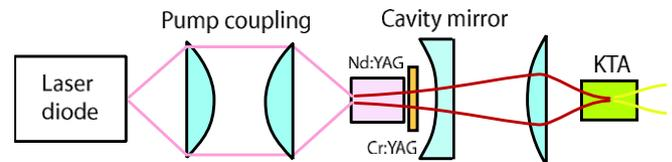
Fig. 1. Schematic figure of the diode-pumped passively Q-switched Nd:YAG/KTA laser.
