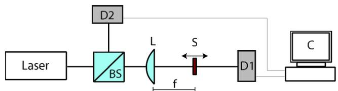
Fig. 6. Setup for measuring the saturation of  $\text{Cr}^{4+}$ :YAG. D1 = power meter for transmitted light, D2 = reference power meter, BS = beam splitter, L = focusing lens, S =  $\text{Cr}^{4+}$ :YAG sample, and C = computer for data logging.
