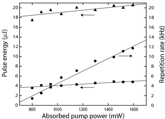
Fig. 3. Repetition rate (●) and pulse energy at 561 nm (■) and 1123 nm (▲) as a function of the absorbed pump power.
