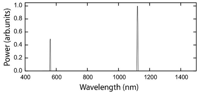
Fig. 5. Measured spectrum of the Nd:YAG/KTA laser.
