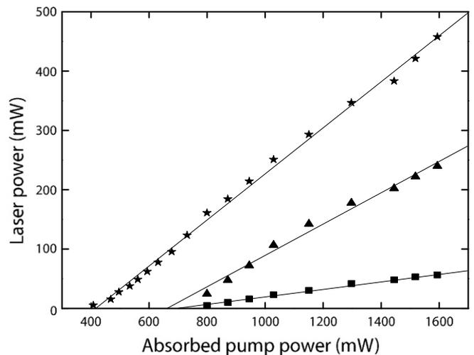
Fig. 2. Laser average power as a function of absorbed pump power for 561 nm Q-switched (■), 1123-nm Q-switched (▲), and 1123 nm CW (★) lasers.
