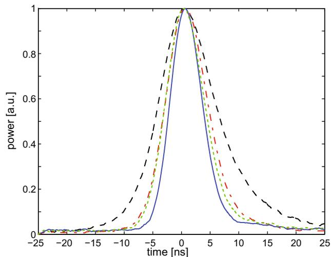
**Fig. 3.** Normalized time traces of the laser pulses at 1123, 561, 374 and 280 nm (dashed, dash dotted, dotted and solid, respectively).
