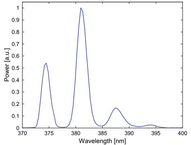
**Fig. 4.** A spectrum of the 374 nm laser after the 30 m of pure silica single mode fiber.
