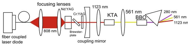
**Fig. 1.** Schematic picture of the setup. For the 374 nm laser the BBO crystal is replaced the BIBO crystal.
