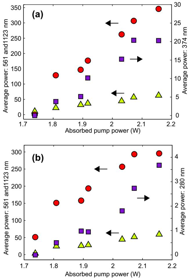
**Fig. 2.** Average laser powers of the a) 374 nm laser and b) 280 nm lasers are presented as a function of the absorbed pump power. In figure a) average power is shown at 1123 nm (circles), 561 nm (triangles) and 374 nm (squares). In figure b) average power is shown at 1123 nm (circles), 561 nm (triangles) and 280 nm (squares).
