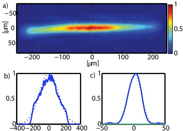
FIG. 3 a) Blue beam intensity at the focus in the BIBO crystal imaged to a beam camera. Measured cross sections (solid) and Gaussian fits (dotted) in the walk-off b) and perpendicular to walk-off c) directions. FWHM beam widths are 283 b) and 27  $\mu\text{m}$  c).
