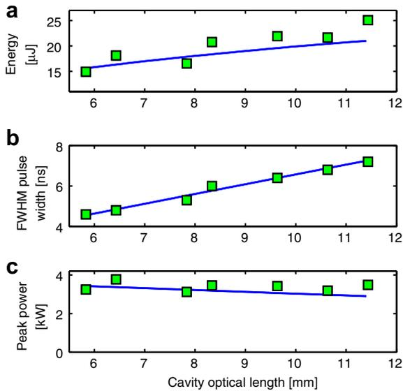
Fig. 3. Pulse parameters as a function of the optical length of the cavity: (a) measured (squares) and calculated values (line) for pulse energy, (b) measured values (squares) and fitted line for pulse length (FWHM) and (c) peak power calculated from data of Figures (a) and (b).
