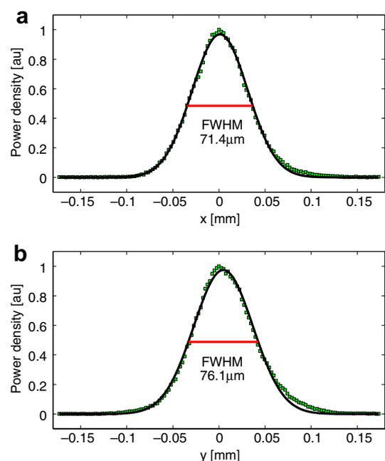
Fig. 4. Beam profiler measurement of the focused beam in  $x$  and  $y$ -directions (squares), Gaussian fit to the data (lines) and FWHM width.
