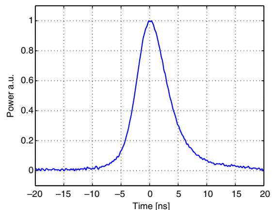
Fig. 2. An oscilloscope trace of a single 946 nm laser pulse.
