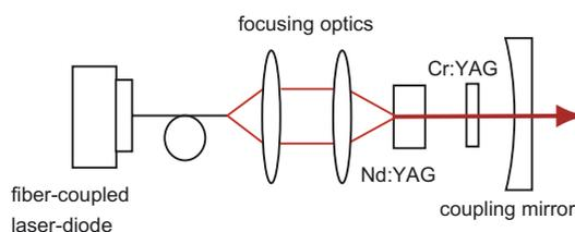
Fig. 1. Schematic picture of the setup.
