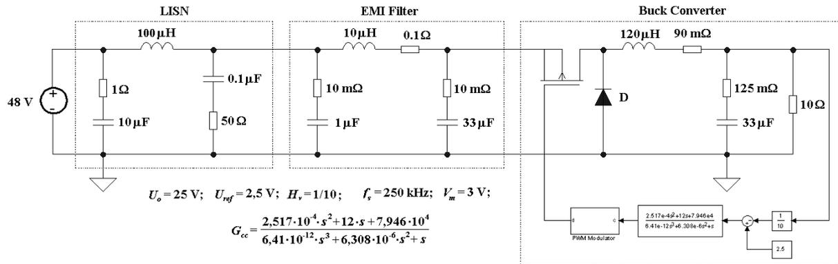
Fig. 7: Values for the components of the VMC buck converter, the EMI filter and the LISN used in the simulations for measuring the insertion loss of the filter.
