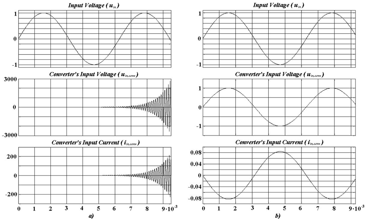
Fig. 5: Simulation of a  $\pi$ -filter with  $C_1 = 33 \mu\text{F}$ ,  $L = 10 \mu\text{H}$  and  $C_3 = 1 \mu\text{F}$ , terminated with  $Z_{in} = -12 \Omega$ .
