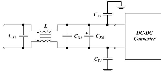
Fig. 1: Typical EMI filter for SMPC [3].
