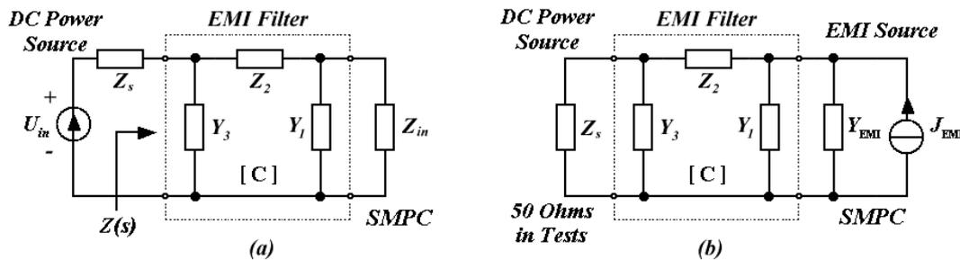
Fig. 4: Circuit to be analysed in: a) stability analysis and b) insertion loss calculations.
