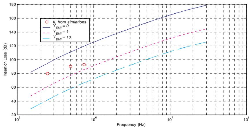
Fig. 8: *IL* of a  $\pi$ -filter, used as input filter of a buck converter.
