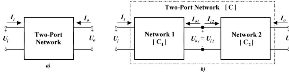
Fig. 2: a) A general two-port network with voltages and currents defined.
