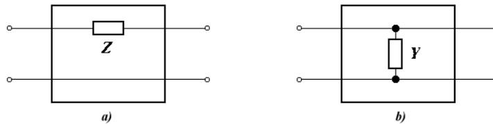
Fig. 3: a) Series connected component; b) parallel connected component.
