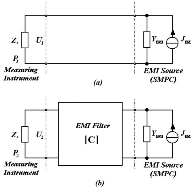
Fig. 6: Definition of the insertion loss.
