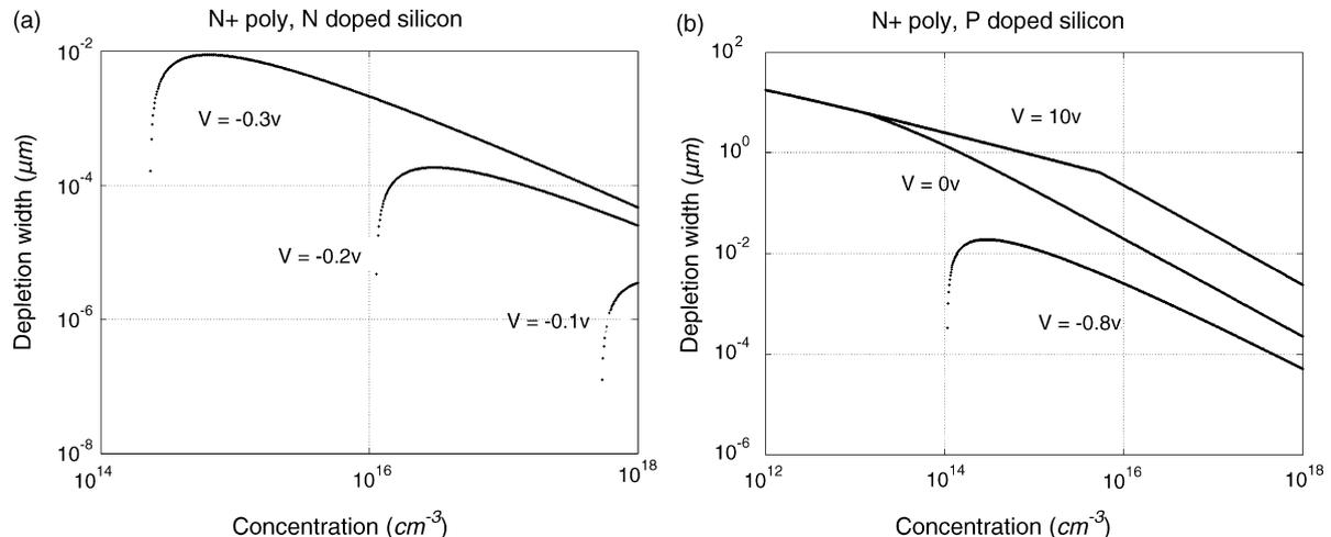
Fig. 8. (a) N+ doped polycrystalline silicon as conductive filling, depletion layer in N type silicon substrate. (b) N+ doped polycrystalline silicon as conductive filling, depletion layer in P type silicon substrate.
