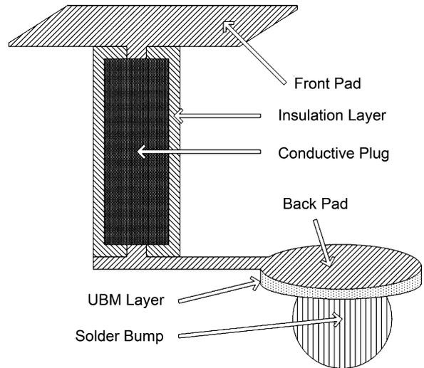
Fig. 1. Test structure design.
