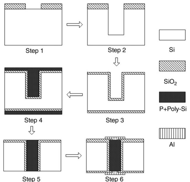
Fig. 2. Processing flow of TWIs' fabrication.
