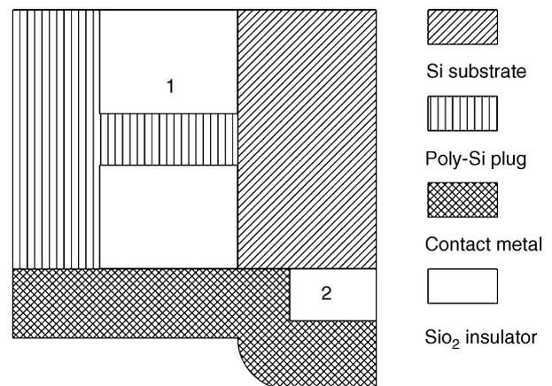
Fig. 11. Possible defect mechanisms on the sidewall of TWI.
