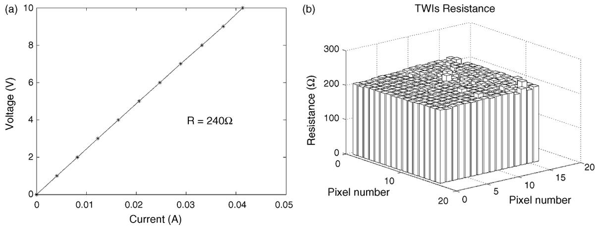
Fig. 9. (a) Individual TWI *I*–*V* curve characteristic. (b) Resistance distribution of TWIs array.
