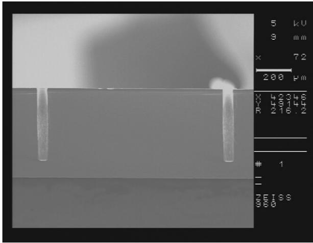
Fig. 4. ICP etching result, the etching depth is pre-set to 420  $\mu\text{m}$  to guarantee that after ICP etching every cavity will reach the target depth.
