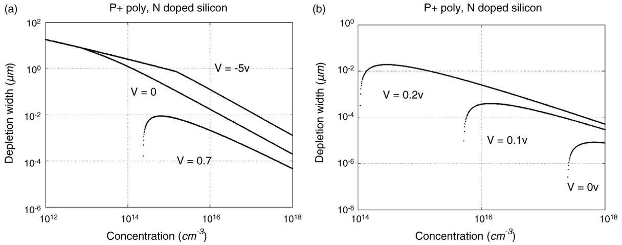
Fig. 7. (a) P+ doped polycrystalline silicon as conductive filling, depletion layer in N type silicon substrate. (b) P+ doped polycrystalline silicon as conductive filling, depletion layer in P type silicon substrate.
