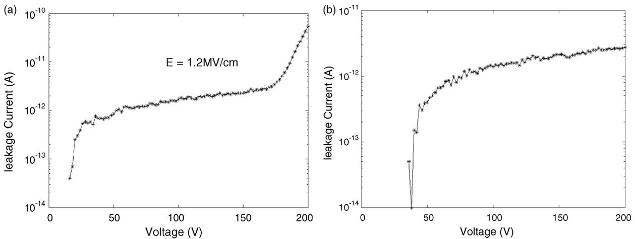
Fig. 10. (a) Leakage current from polycrystalline silicon plug to silicon substrate. (b) Leakage current between two adjacent TWIs.
