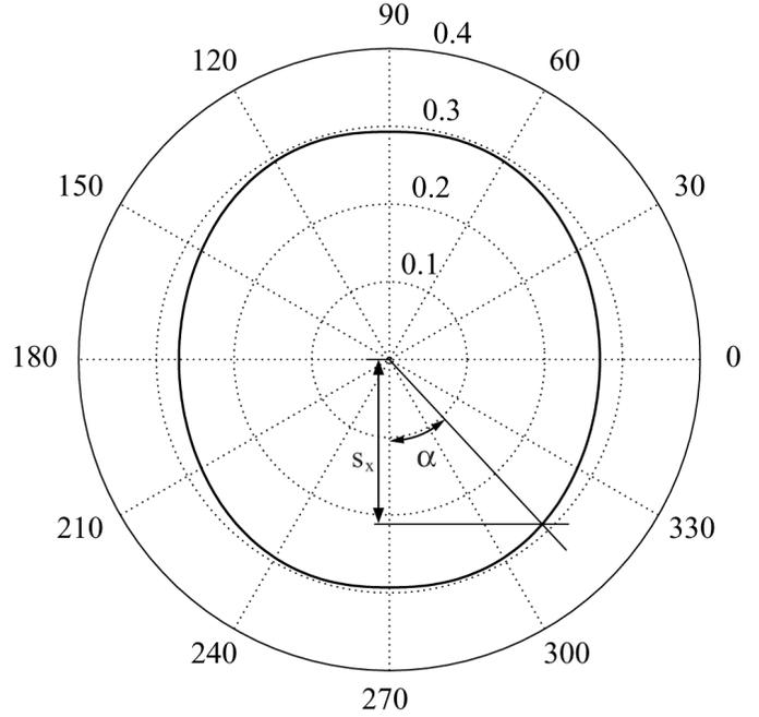
Fig. 6. Rayleigh SAW slowness (in  $10^{-3}$  s/m) for Y-cut  $\text{LiNbO}_3$  as a function of the propagation direction  $\theta$  on the shorted substrate surface.  $s_x$  is the  $x$  component of the surface slowness, and it is parallel with the crystallographic  $Z$  axis.
