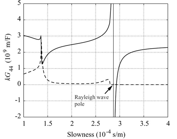
Fig. 2. Scaled component  $G_{44}$  for  $\text{YZ-LiNbO}_3$  [Euler angles:  $(0^\circ, -90^\circ, -90^\circ)$ ]. The propagation direction of the wave is along the positive  $Z$  axis of the crystal. Solid and dashed curves are the real and imaginary parts, respectively.
