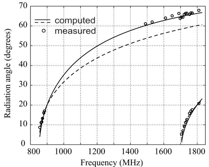
Fig. 10. Experimental and theoretical angles of radiation versus frequency for Rayleigh SAW emanating from LLSAW resonator on YZ-LiNbO<sub>3</sub>. The solid line is the computed direction of the energy flow (group velocity) and dashed line is the computed direction of the wave vector (phase velocity), both for shorted surface.
