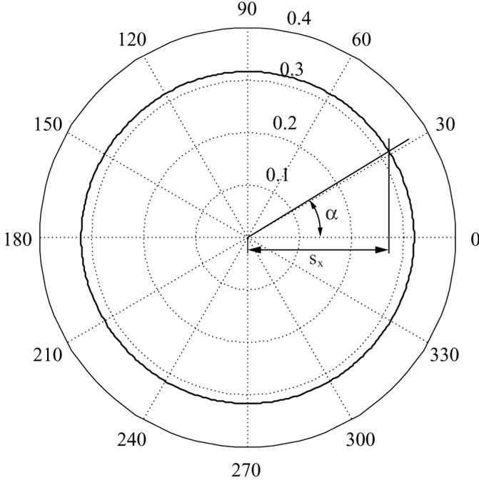
Fig. 5. Rayleigh SAW slowness (in  $10^{-3}$  s/m) for  $42^\circ$ Y-cut  $\text{LiTaO}_3$  as a function of the propagation direction  $\theta$  on the shorted substrate surface.  $s_x$  is the  $x$  component of the surface slowness, and it is parallel with the crystallographic  $X$  axis.
