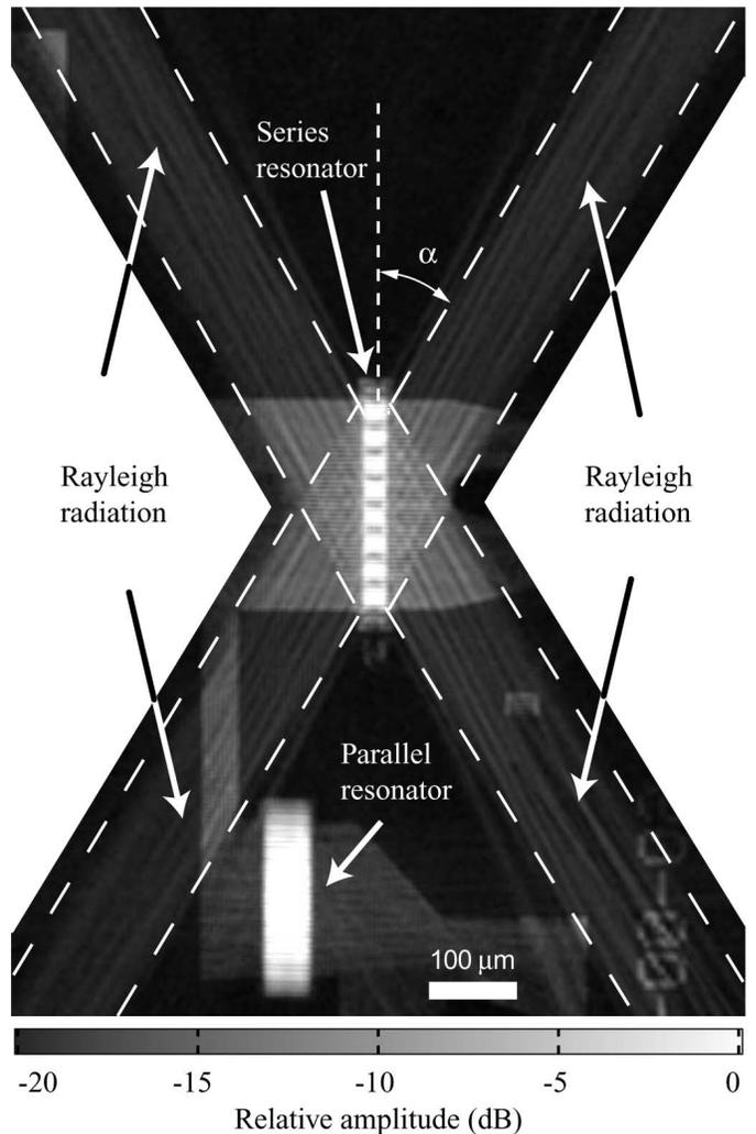
Fig. 3. X-shaped Rayleigh SAW radiation pattern emitted from a series impedance element of a LSAW ladder filter on  $42^\circ\text{YX-LiTaO}_3$ . The resonator is aligned along the crystallographic  $X$  axis (vertical direction in the figure). Note that the sensitivity of the interferometer is different on crystal, on metal, and on grating. Note also the weak Rayleigh-wave beam propagating in the direction perpendicular to the parallel resonator.
