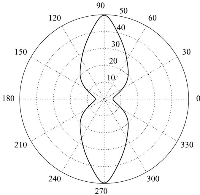
Fig. 8. Rayleigh SAW coupling strength,  $\Gamma$ , on the free surface of Y-cut LiNbO<sub>3</sub> (in  $10^6$  m/F) as a function of the propagation direction  $\theta$ .
