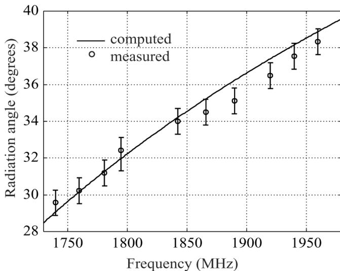
Fig. 9. Experimental and theoretical angles of radiation versus frequency for Rayleigh SAW emanating from LSAW resonator on 42°YX-LiTaO<sub>3</sub>.
