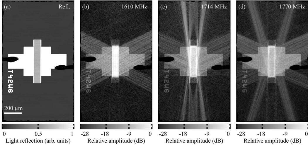
Fig. 4. Selected laser-interferometric scans of the LLSAW resonator on YZ-LiNbO<sub>3</sub> (the resonator is aligned along the crystallographic  $Z$  axis). (a) Light-reflection image, i.e., light reflectivity of the surface, and relative amplitudes of the vertical vibration component at the frequency (b) 1610 MHz, (c) 1714 MHz, and (d) 1770 MHz. Note that the sensitivity of the interferometer is different on crystal, on metal, and on grating.
