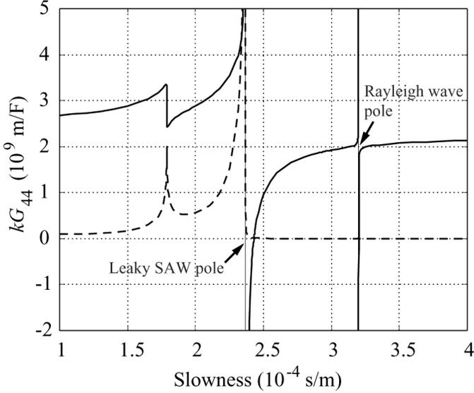
Fig. 1. Scaled component  $G_{44}$  for  $42^\circ\text{YX-LiTaO}_3$  [Euler angles:  $(0^\circ, -48^\circ, 0^\circ)$ ]. The propagation direction of the wave is along the positive  $X$  axis of the crystal. Solid and dashed curves are the real and imaginary parts, respectively.
