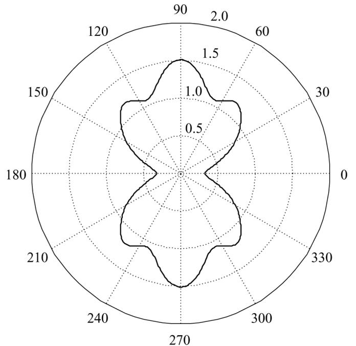
Fig. 7. Rayleigh SAW coupling strength,  $\Gamma$ , on the free surface of  $42^\circ$ Y-cut  $\text{LiTaO}_3$  (in  $10^6$  m/F) as a function of the propagation direction  $\theta$ .
