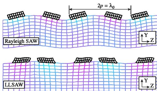
FIG. 1. (Color online). Schematic view of the Rayleigh SAW and LLSAW displacements. Both waves have displacement components in  $(Y, Z)$  plane, but for the LLSAW, the  $Z$  component is dominating. The displacements are greatly exaggerated.
