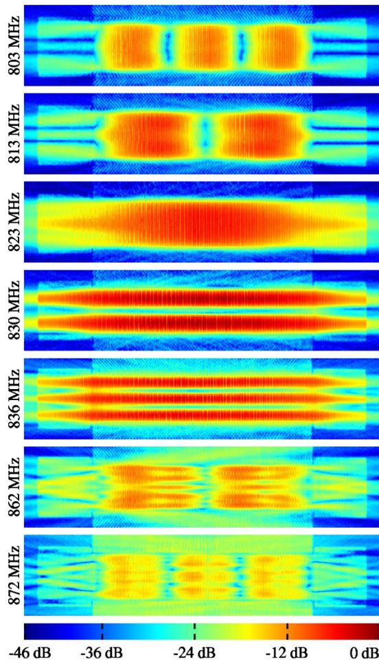
FIG. 3. (Color online). Relative amplitudes of the vertical displacement component at selected frequencies for the Rayleigh waves. Below the resonance frequency (823 MHz), the longitudinal profile possesses a typical beating pattern. Above the resonance, transversal modes are observed.
