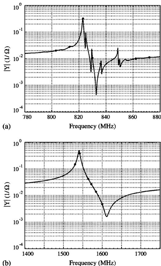
FIG. 2. Measured magnitude of the admittance as a function of frequency for (a) the Rayleigh mode and (b) the LLSAW mode. The dots indicate the frequencies for which the measured profiles are presented. The electrical response of the resonator is measured directly on the chip in 50  $\Omega$  environment.
