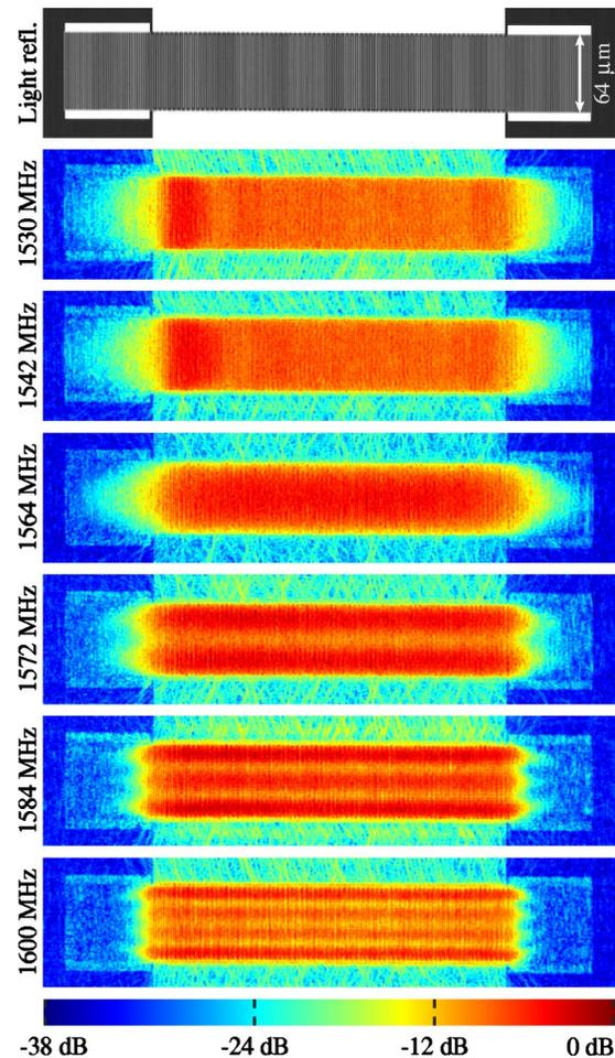
FIG. 4. (Color online). Relative amplitudes of the vertical displacement component at selected frequencies for the LLSAW. In the light reflection image, white areas represent aluminum coating and black areas, LiNbO<sub>3</sub> crystal. The beating pattern, present for Rayleigh waves in Fig. 3, is not observed here. Transversal structure appears above the resonance frequency.
