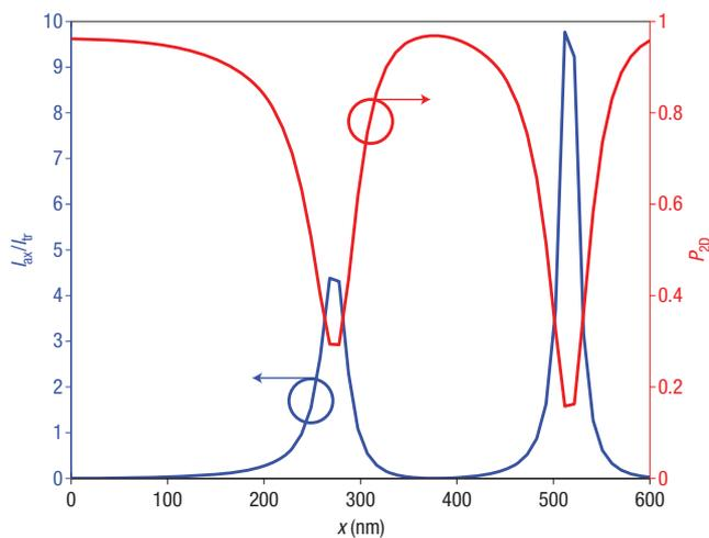
**Figure 5** Influence of the axial electric-field component on  $P_{2D}$ . The theoretically calculated ratio of the intensities of the electric-field components along  $I_{\text{ax}}$  and perpendicular  $I_{\text{tr}}$  to the optical axis (blue curve) and the degree of polarization  $P_{2D}$  (red curve) are shown for the cut (j) of Fig. 4f.
