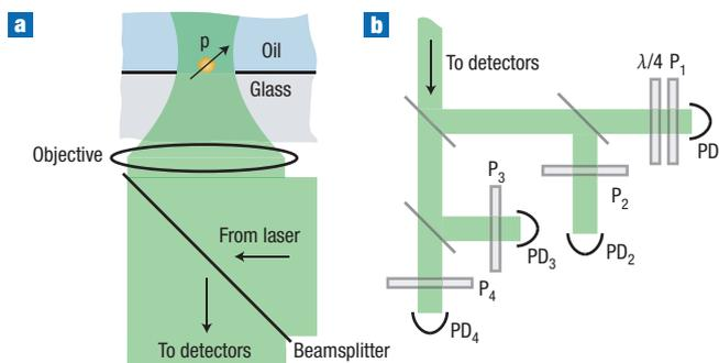
**Figure 2** Experimental set-up for mapping the degree of polarization.
