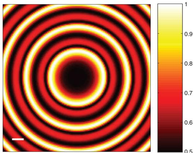
**Figure 1** Distribution of  $P_{3D}$  in the focal plane of a high-NA lens. The incident light (wavelength 532 nm) is an unpolarized plane wave ( $P_{2D} = 0$ ; note that in the three-dimensional representation such waves have  $P_{3D} = 0.5$ ; refs 16 and 17). The NA of the lens is 1.3 and the refractive index in the focal region is 1.5. The scale bar represents 100 nm. The coloured scale represents  $P_{3D}$ .
