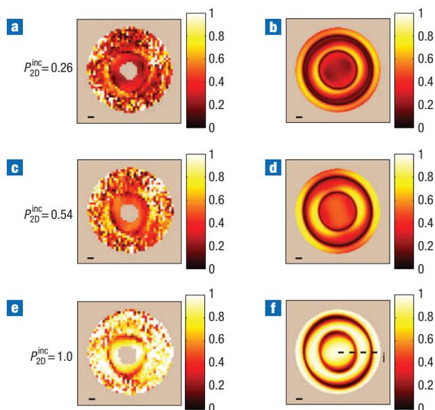
**Figure 4** Measured  $P_{2D}$  for different values of the degree of polarization of the incident beam  $P_{2D}^{\text{inc}}$ . **a,c,e**, Experimental observations. **b,d,f**, Corresponding theoretical predictions. In **a** and **b**  $P_{2D}^{\text{inc}} = 0.26$ ; in **c** and **d**,  $P_{2D}^{\text{inc}} = 0.54$ , and in **e** and **f**,  $P_{2D}^{\text{inc}} = 1.0$ . All scale bars are 100 nm. All the coloured scales represent  $P_{2D}$ .
