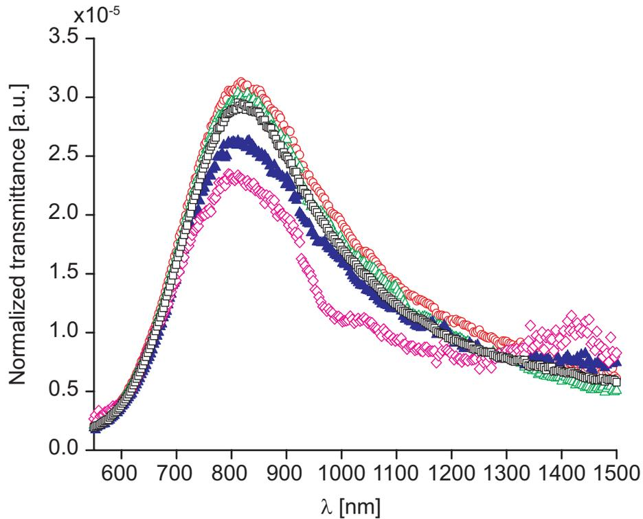
Fig. 5. Transmission spectra of 33 nm wide slits in 193 nm thick gold film for different slit lengths: 25  $\mu\text{m}$  (black open squares), 10  $\mu\text{m}$  (red open circles), 5  $\mu\text{m}$  (green open triangles), 2.5  $\mu\text{m}$  (blue solid triangles), and 1.25  $\mu\text{m}$  (magenta diamonds). The spectra were normalized with the slit length in micrometers. The polarization of the incident light is orthogonal to the slit ( $\theta = 0^\circ$ , see Fig. 1).
