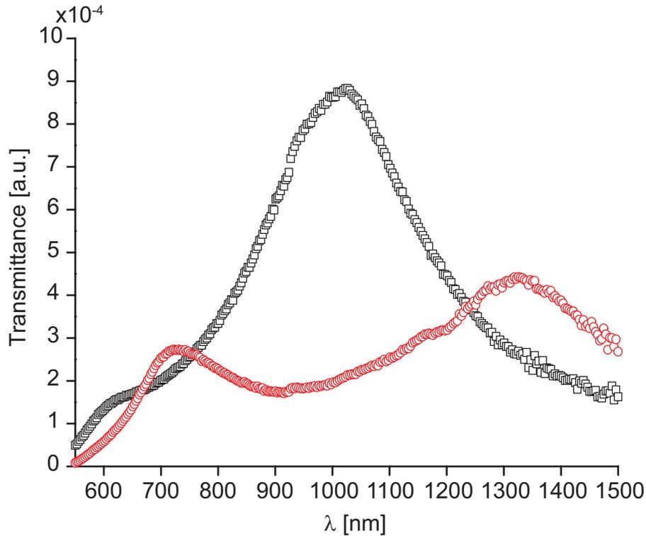
Fig. 8. Change in transmission spectrum when a drop of 1,9-nonanedithiol is applied to the sample: transmission spectrum of a 26 nm wide slit milled in a 270 nm thick gold film for air (black open squares) and 1,9-nonanedithiol (red open circles) in the slit.
