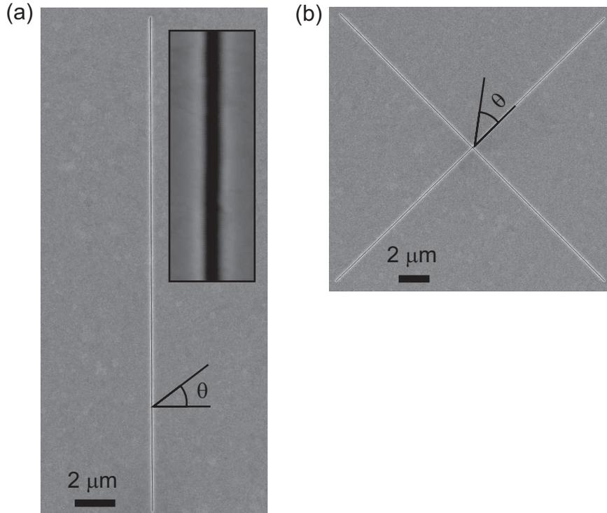
Fig. 1. Scanning electron micrographs of nanoslits fabricated in gold film by focused ion beam milling: (a) 33 nm wide slit and (b) 31 nm linewidth cross. The inset in (a) displays a section of the slit at higher magnification. The angle  $\theta$  in (a) and (b) defines the direction of polarization of the incident field.
