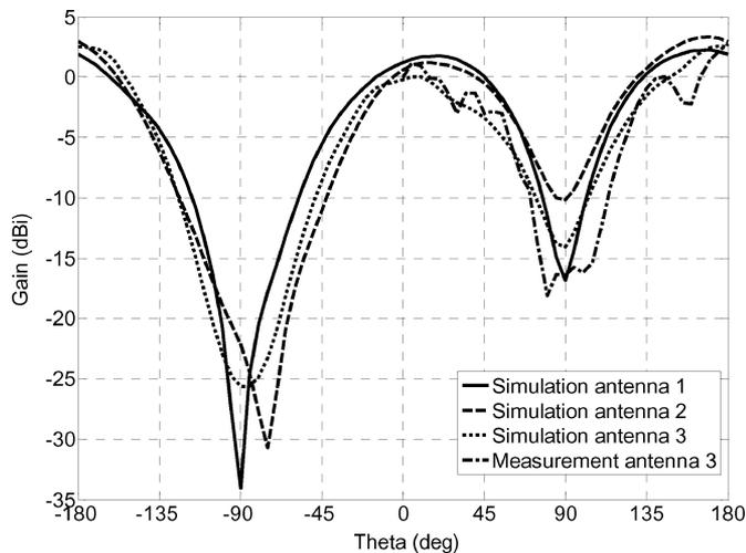
Fig. 5. Simulated and measured gain in the  $y$ - $z$  plane at 60.5 GHz.
