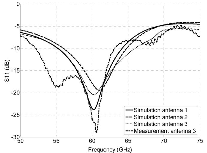
Fig. 3. Simulated and measured return loss.
