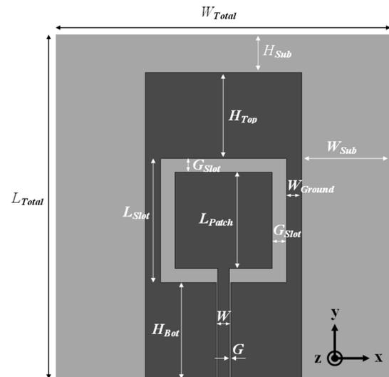
Fig. 1. Layout of the antenna.
