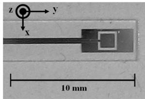
Fig. 2. Picture of the measured antenna with part of the feed line.
