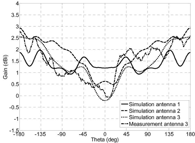
Fig. 4. Simulated and measured gain in the  $x$ - $z$  plane at 60.5 GHz.
