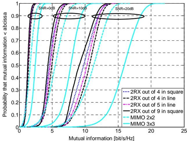
Fig. 6. MI obtained by selecting 2RX out of  $N$ , with the SNR criterion and the realistic switching network.
