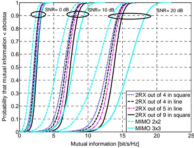
Fig. 3. MI obtained by selecting 2 RX out of  $N$ , with optimum capacity criterion and the ideal switching network.
