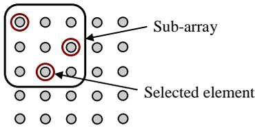
Fig. 2. Example of 3 selected antennas out of a sub array of 9 elements in square.
