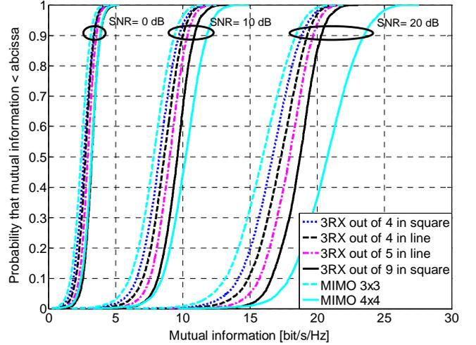
Fig. 4. MI obtained by selecting 3 RX out of  $N$ , with the optimum capacity criterion and the ideal switching network.
