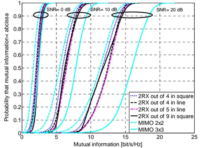
Fig. 5. MI obtained by selecting 2 RX out of  $N$ , with the SNR criterion and the ideal switching network.
