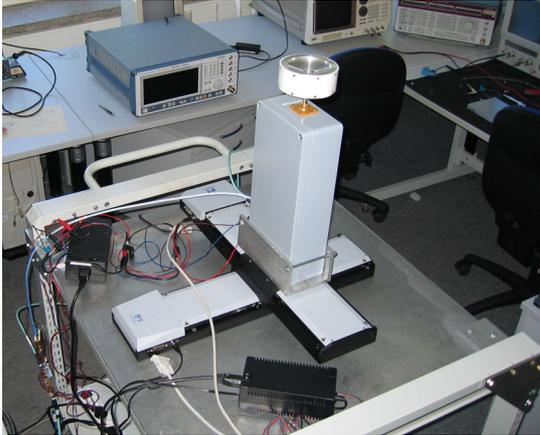
Fig.2. Picture of the transmitter (up converter and antenna) on the scanner.
