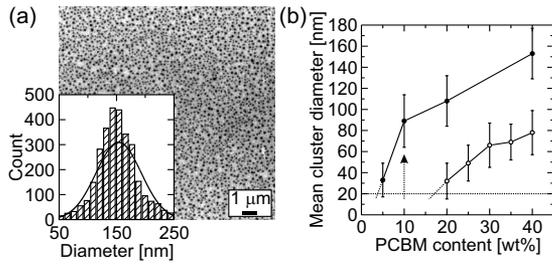
FIG. 2. (a) Size distribution for 120 °C annealed 40 wt % PCBM/PS. (b) Mean cluster diameters in PCBM/PS thin films before (open symbols) and after thermal annealing at 120 °C (closed symbols) as determined from the TEM micrographs. The error bars indicate the standard deviation and the smallest detectable particle size is ca. 20 nm.
