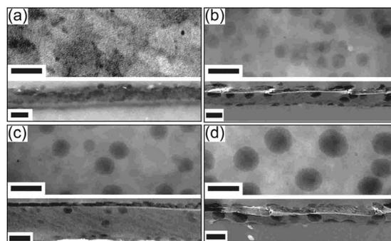
FIG. 1. TEM micrographs showing the plan view (top) and cross-sectional view (bottom) for 120 °C annealed (a) 5 wt %, (b) 10 wt %, (c) 20 wt %, and (d) 40 wt % PCBM/PS thin films. The top interfaces in the cross sections are air/film and the bottom film/substrate interfaces. All scale bars are 200 nm.
