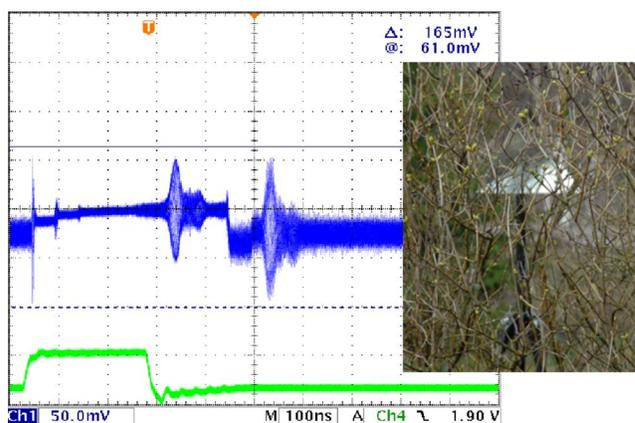
FIG. 5. (Color online) Recorded radar response from the target placed behind a road-side bush. The attenuation is 10–13 dB/m. The upper trace is the detected signal. The first pulse is the transmitted signal leaking through the circulator. Lower trace is the signal used to trigger the oscilloscope.
