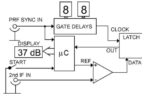
FIG. 3. Block diagram of the gated comparator level measuring system.
