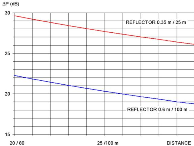
FIG. 1. (Color online) Available dynamic range with two different antennas against perpendicular surface clutter from foliage. Target RCS is 20 dBsm.
