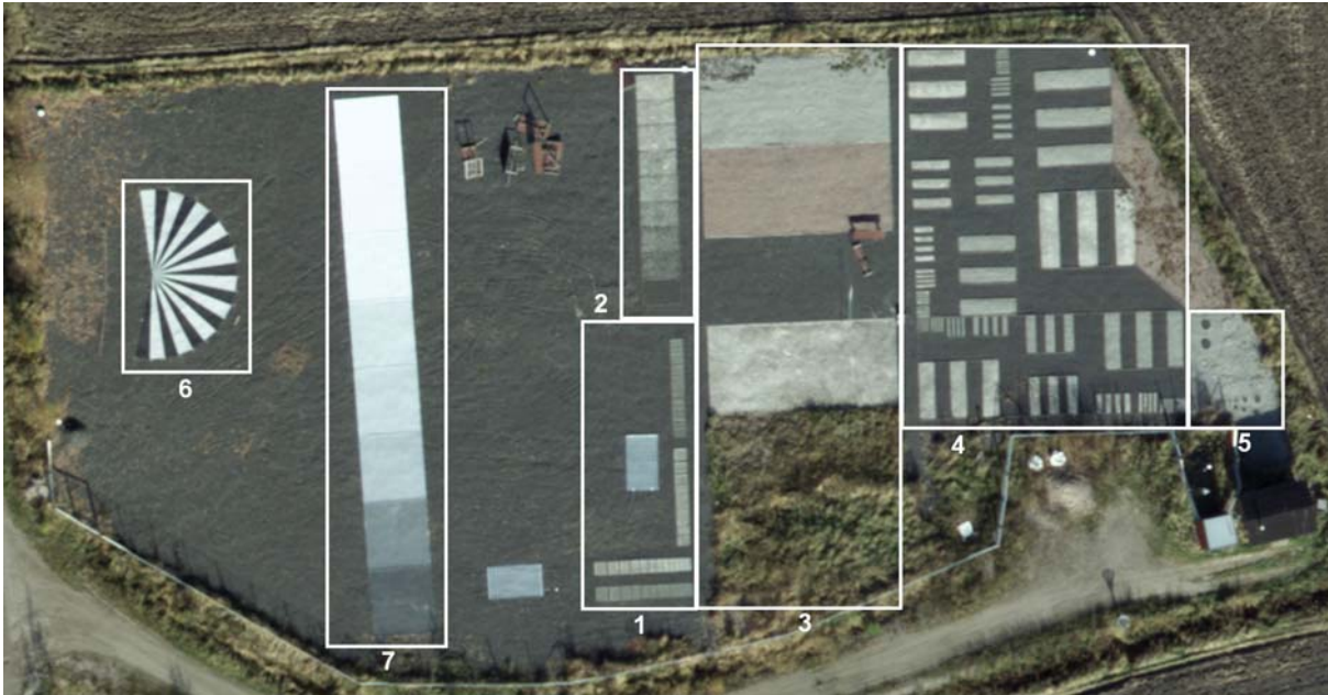
Figure 7. The Sjökkulla image quality test field: 1) permanent dense resolution bar target, 2) permanent gray scale, 3) permanent reflectance targets, 4) sparse resolution bar target, 5) permanent circular targets, 6) portable Siemens star, and 7) portable gray scale.
