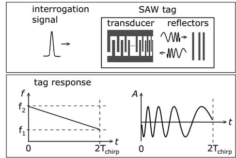
Fig. 5. Interrogation of SAW tag with a delta pulse.
