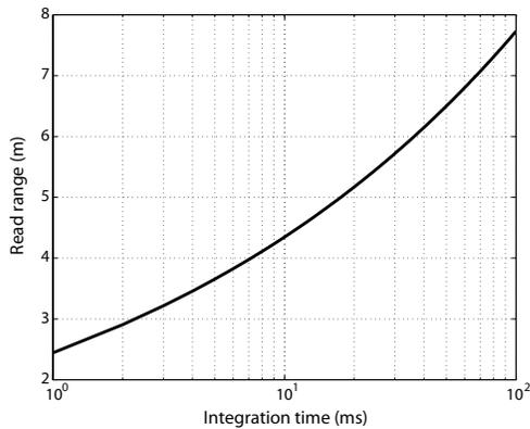
Fig. 16. Estimated read range  $r$  as a function of reader integration time  $T_i$  for a 2.25-GHz UWB SAW tag satisfying the FCC rules.
