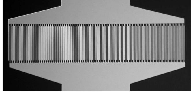
Fig. 12. Chirp transducer of fabricated SAW tag device. Aperture is  $75 \mu\text{m}$  and length is  $400 \mu\text{m}$ . Critical dimension is  $0.77 \mu\text{m}$ . Center frequency is 1 GHz.
