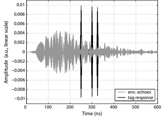
Fig. 4. Real parts of the tag response and the environmental echoes after being processed with a dispersive delay line matched to the tag response. Matlab simulation.
