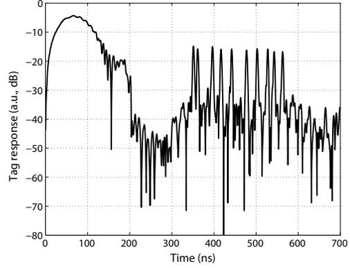
Fig. 14. Compressed response of a SAW tag device having 10 code reflectors. Simulated data.
