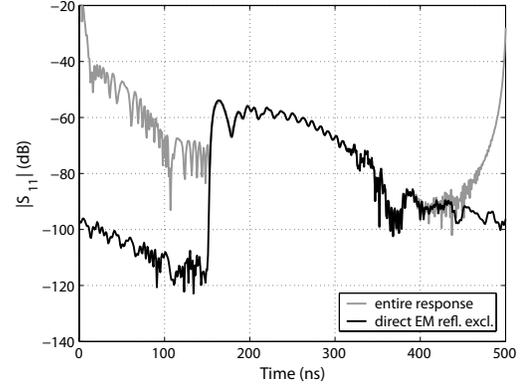
Fig. 8.  $|S_{11}|$  in the time domain for the entire single-reflector SAW tag device and for the case where the direct EM reflection from the transducer has been excluded. FEM-BEM simulation.
