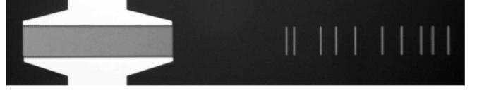
Fig. 11. Fabricated SAW tag device. Structure length is 1.1 mm.
