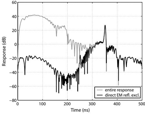
Fig. 10. Tag responses of Fig. 9 after compression by an ideal up-chirp correlator.
