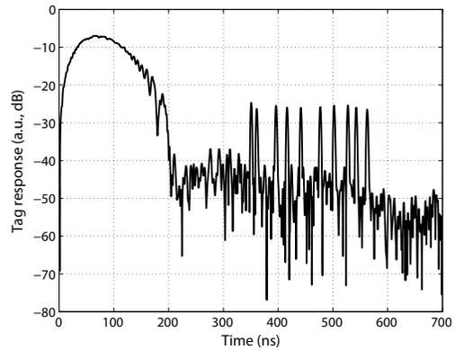
Fig. 15. Compressed response of a SAW tag device having 10 code reflectors. Experimental data.
