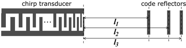
Fig. 1. A schematic drawing of a SAW tag consisting of a chirp transducer and an array of wide-band code reflectors.
