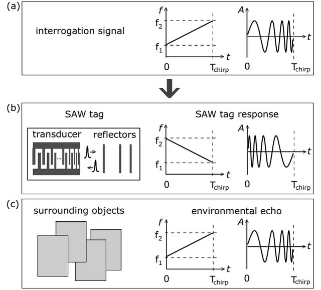
Fig. 2. Interrogation process. (a) An up-chirp LFM signal is used for interrogation. (b) The signal is compressed by the chirp transducer, reflected by the code reflectors, and expanded by the transducer. The output has a dispersion opposite to that of the interrogation signal. (c) Reflections from surrounding objects have the same dispersion as the interrogation signal.
