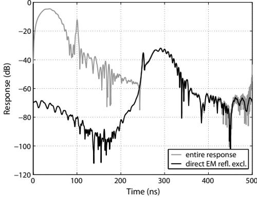
Fig. 9. Tag response to an up-chirp signal for the entire single-reflector SAW tag device and for the case where the direct EM reflection from the transducer has been excluded. FEM-BEM simulation.
