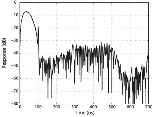
Fig. 13. Tag response to an up-chirp interrogation signal. The response contains 10 overlapping chirped code reflections between 250 ns and 550 ns. Experimental data.
