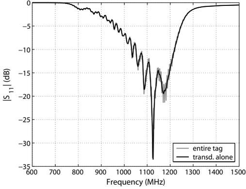
Fig. 6.  $|S_{11}|$  in the frequency domain for the entire single-reflector SAW tag device and for the chirp transducer alone. FEM-BEM simulation.
