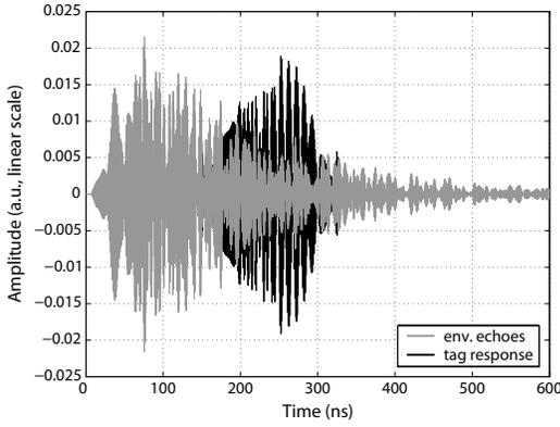
Fig. 3. Real parts of the tag output and the environmental echoes. Matlab simulation.
