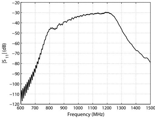
Fig. 7.  $|S_{11}|$  in the frequency domain for the single-reflector SAW tag device after subtraction of the signal directly reflected from the chirp transducer. FEM-BEM simulation.
