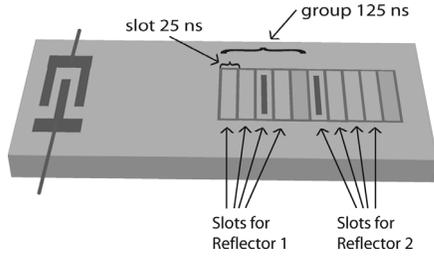
Fig. 1. SAW tag based on time position encoding.
