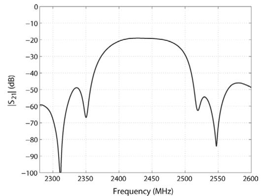
Fig. 7.  $|S_{21}|$  for a Z-path delay line consisting of two identical SPUDTs separated by a Z-path and having an acoustic path length of about  $3.8\ \text{mm}$ . Experimental data.
