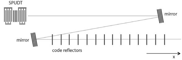
Fig. 5. Z-path geometry.
