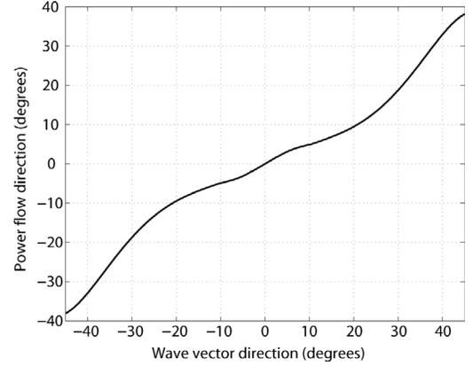
Fig. 11. Power flow direction  $\theta_e$  versus wave vector direction  $\theta$  for  $128^\circ$ -LiNbO<sub>3</sub>.
