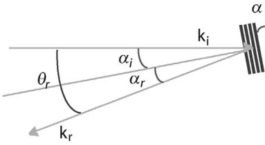
Fig. 8. Reflection of the wave vector at the first mirror.
