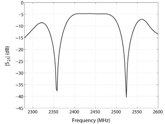
Fig. 6.  $|S_{21}|$  for an inline delay line consisting of two identical SPUDTs facing each other and separated by  $300\ \mu\text{m}$ . Simulation.
