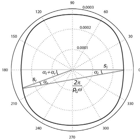
Fig. 9. Phase slowness  $s$  versus wave vector direction  $\theta$  for  $128^\circ$ -LiNbO<sub>3</sub>. ( $s$  is in seconds/meter and  $\theta$  in degrees.)
