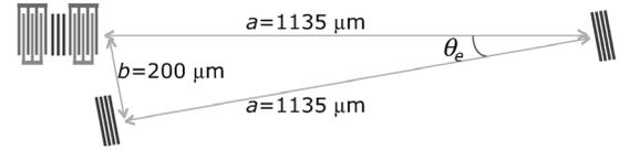
Fig. 12. Power flow direction and distances determining the mirror positions.
