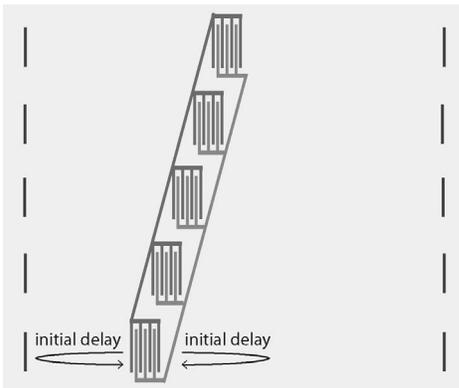
Fig. 3. SAW tag having a multichannel geometry.
