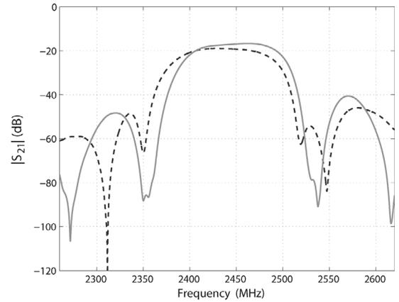
Fig. 15.  $|S_{21}|$  for a Z-path delay line. Original (dashed) and improved (solid) designs. Experimental data.
