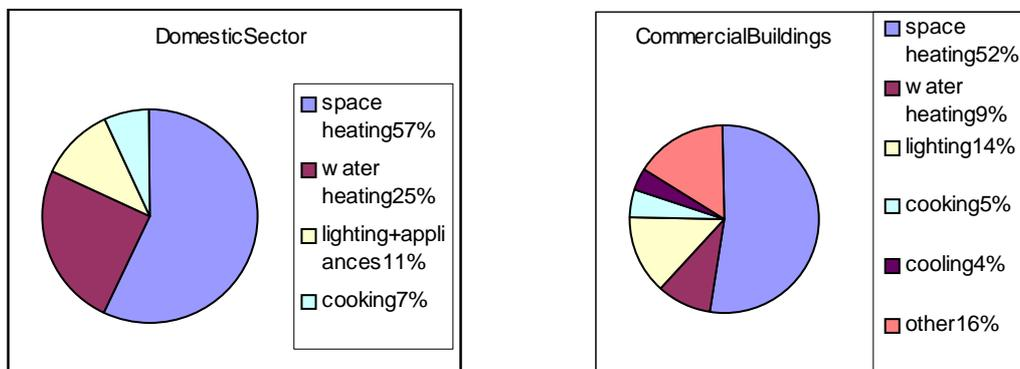
Figure 2 Energy consumption by end use in the EU domestic and commercial buildings [EC 2007]
