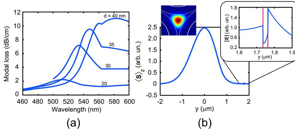
Fig. 2. (a) Modal loss  $\alpha$  as a function of wavelength for different gold layer thicknesses  $d$ . (b) Longitudinal component of the time-averaged Poynting vector,  $\langle \mathbf{S} \rangle_z$ , on the  $y$ -axis. Left inset: cross-sectional view of the mode profile. Right inset: close-up of the norm of the electric field with the vertical lines marking the gold layer location.
