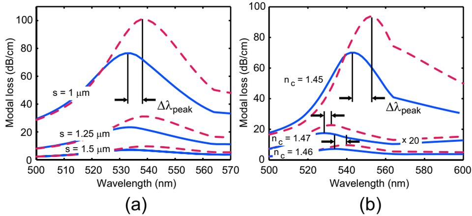
Fig. 3. Modal loss as a function of wavelength for two analytes with refractive indices  $n_a = 1.33$  (solid) and  $n_a = 1.34$  (dashed). The curves are plotted for (a) different dielectric layer thicknesses  $s$  and (b) different refractive indices  $n_c$  of the core. In (b), the data for  $n_c = 1.47$  are magnified by a factor of 20 for clarity.
