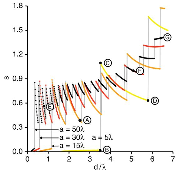
Fig. 4. (Color online) Parameter  $s = \sigma z_T$  as a function of the normalized core thickness  $d/\lambda$ . The gray curves connect the data points corresponding to a certain value of the core radius  $a$ . The points labeled with the uppercase letters correspond to the cases of Fig. 5.
