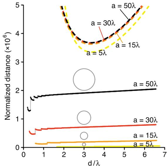
Fig. 3. (Color online) Normalized Talbot distance  $z_T k$  (dots connected with gray curve) and the beat length  $z_B k$  (dashed curve) of the modes  $TE_{0,1}$  and  $TM_{0,1}$  as a function of the normalized core thickness  $d/\lambda$  for four different values of the inner radius of core  $a$ . The relative sizes of the fiber cores are depicted by gray circles for  $d/\lambda = 3$ .
