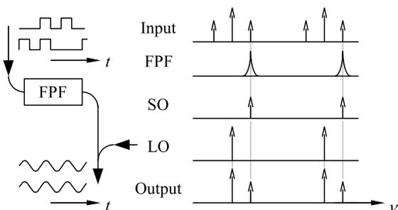
Fig. 1. Multiwavelength clock recovery with optical sideband filtering and heterodyne beating. Abbreviations: FPF – Fabry-Perot filter; SO – signal oscillator; LO – local oscillator.
