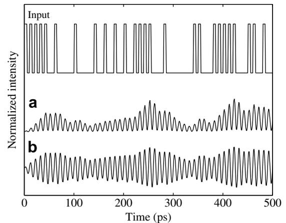
Fig. 2. Simulation of (a) conventional FPF filtering and (b) heterodyne beats of sideband-filtered signal. Simulated RZ modulated data rate is 100 Gbit/s, and photon lifetime of the resonator is 31.6 ps (FWHM bandwidth of 5 GHz). The simulation begins with a start-up sequence of five digital ones.
