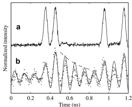
Fig. 4. (a) Input signal and (b) sideband-filtered heterodyne beat. The simulated response (continuous line) follows closely the recorded output (dots). Signal decay envelope (dashed line) has twofold time constant (240 ps) compared to the resonator photon lifetime (120 ps).
