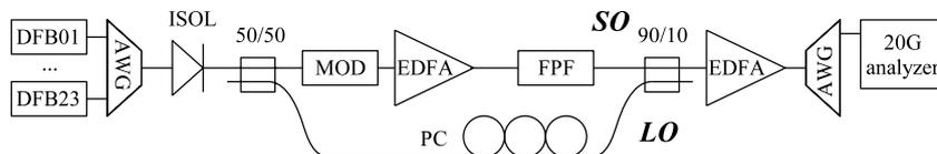
Fig. 3. Experimental setup. Abbreviations: DFB – distributed feedback laser; AWG – arrayed waveguide grating; ISOL – isolator; 50/50 – fiber coupler; MOD – modulation (including RZ pulse shaping and data modulation (see text); EDFA – erbium doped fiber amplifier; FPF – Fabry-Perot filter; PC – polarization controller; SO – signal oscillator; LO – local oscillator; 90/10 – fiber coupler.
