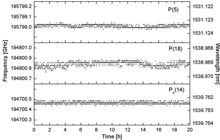
Fig. 6. Frequency stability of laser locked to P(5) of  $^{12}\text{C}^{13}\text{CH}_2$ , P(18) of  $^{12}\text{C}^{13}\text{CH}_2$  and  $\text{P}_e(14)$  of the  $\nu_1 + \nu_3 + \nu_4^1 - \nu_4^1$  transition of  $^{12}\text{C}_2\text{H}_2$  lines of acetylene for 20 h.
