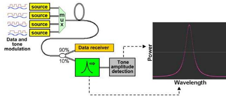
Fig. 1. Operating principle of the monitoring device.
