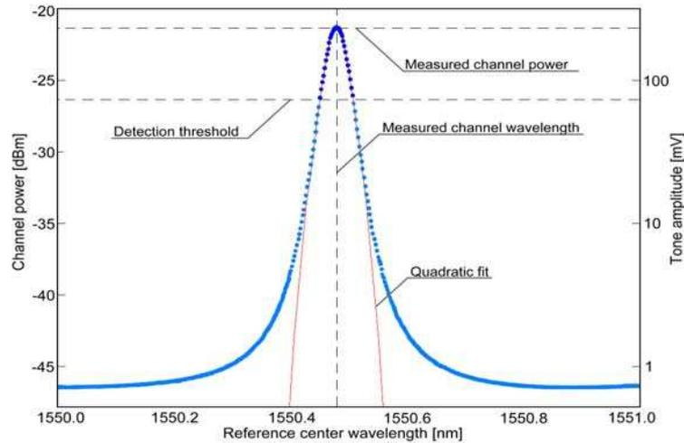
Fig. 2. Extracting the wavelength and power level from the measured data.
