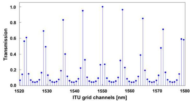
Fig. 6. The attenuating effect of the etalon with a FSR of 110 GHz to the 100-GHz-spaced WDM channels and their respective tones.
