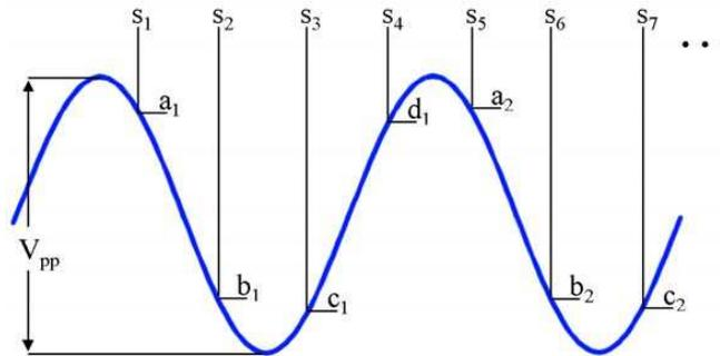
Fig. 4. Principle of the sampling system implemented in the monitoring device.
