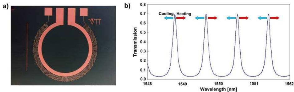
Fig. 3. (a) Microscope image of the silicon etalon showing the two temperature controlling resistors on the etalon surface. (b) Part of the transmission spectrum of the etalon at  $1.55\ \mu\text{m}$ , showing four fringes and their temperature tuning.
