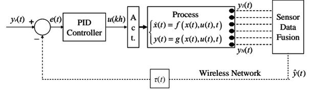
Fig.1. Wireless networked control system.
