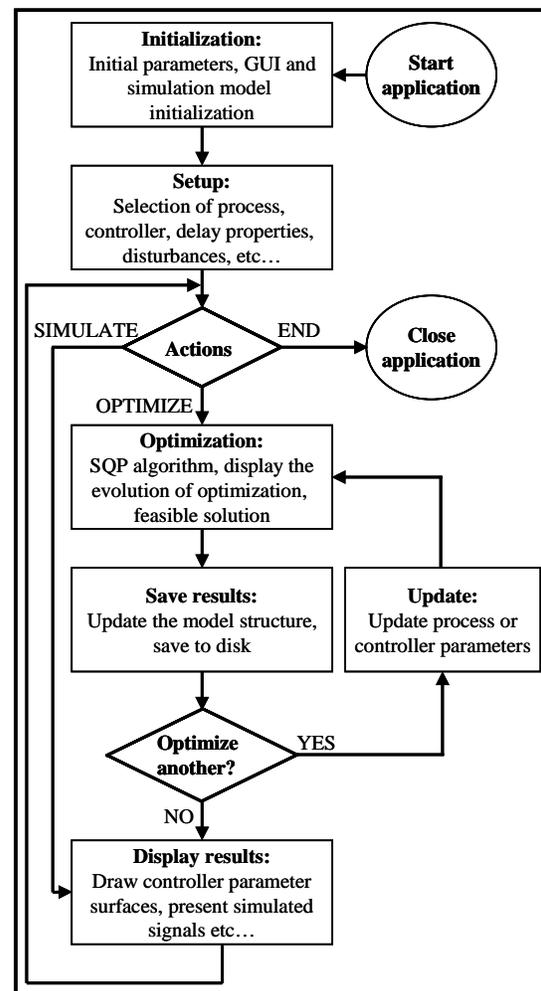
Fig.4. Program execution phases of the tuning tool.
