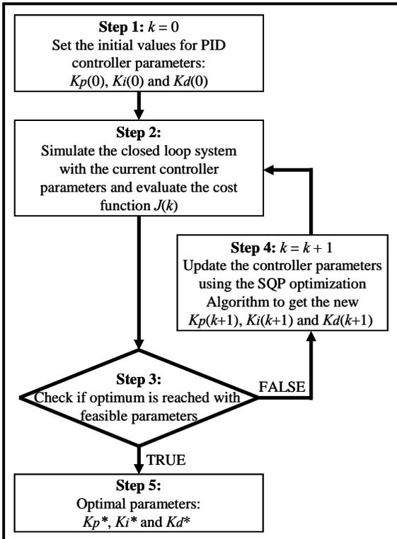
Fig.2. Optimal PID tuning (modified from [11]).
