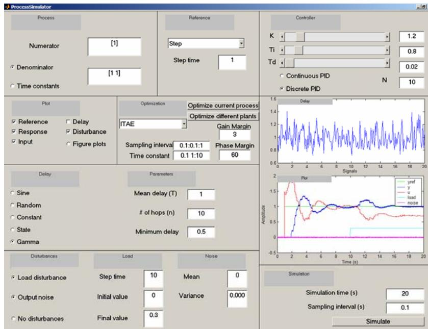
Fig.3. The PID controller tuning tool – GUI.
