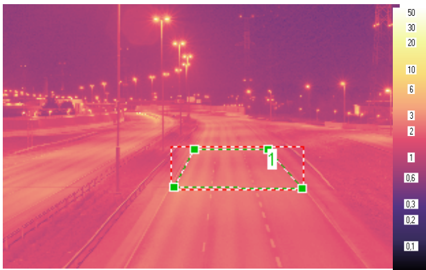
Fig. 10. Luminance distributions measured on VT7 in Finland. The road section is lit with 250W HPS lamps. Average luminance L_{av} , overall luminance uniformity U_0 , and longitudinal luminance uniformities for the left U_{L,left} , and right U_{L,right} lanes.
