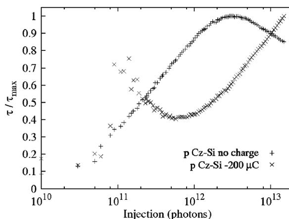
Fig. 3. The injection level dependence in p-type 2 kΩ cm Cz-Si. The both wafer surfaces were negatively charged during the measurement with deposited surface charge.
