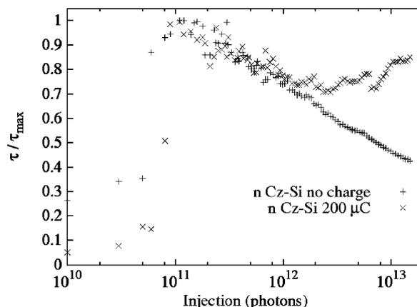
Fig. 1. The injection level dependence in n-type Cz-Si.
